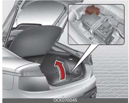
Battery box fuse panel
