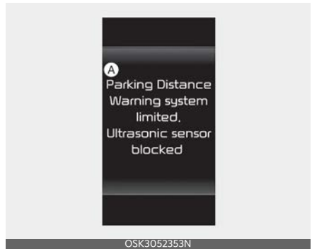
A: Parking Distance Warning system limited. Ultrasonic sensor blocked
