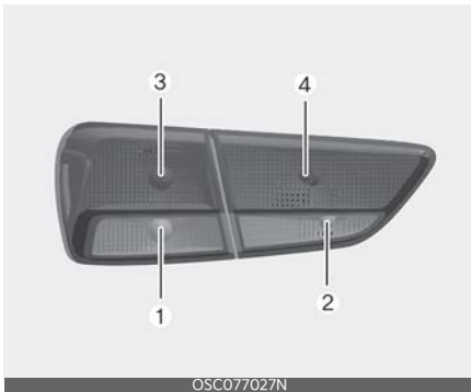
Rear combination lamp (4 Door) - Type A
