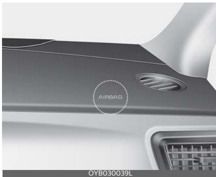
Passenger's front air bag
