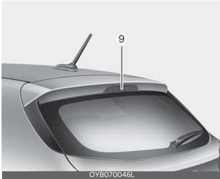
High mounted stop lamp (5 Door)
