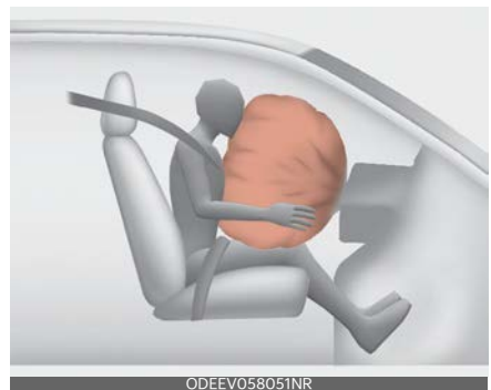
Passenger's front air bag
