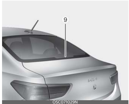
High mounted stop lamp (4 Door)
