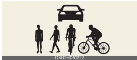
The illustration above shows the image the front view camera and front radar are capable of detecting as a vehicle, pedestrian and cyclist.
