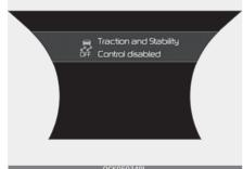
To cancel ESC operation, press the ESC OFF button (ESC OFF <sup>2</sup>/<sub>2</sub>) for more than 3 seconds. ESC OFF indicator light (ESC OFF <sup>2</sup>/<sub>2</sub>) illuminates and ESC OFF warning chime will sound. At this state, the engine control function and brake control function do not operate. It means the car stability control function does not operate any more.
