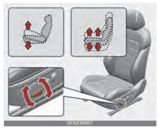
Pull the front portion of the control switch up to raise or press down to lower the front part of the seat cushion. Pull the rear portion of the control switch up to raise or press down to lower the seat cushion. Release the switch once the seat reaches the desired position.
