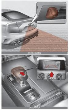
Rear View Monitor will show the area behind the vehicle to assist you when parking or backing up.
