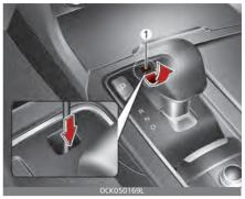
You can move the shift lever, when the battery is discharged. However, it will not change the gear from P (Parking) to N (Neutral) or others.
