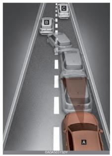
[A]: Your vehicle, [B]: Lane changing vehicle, [C]: Same lane vehicle When driving in stop-and-go traffic, and a stopped vehicle in front of you merges out of the lane, FCA may not immediately detect the new vehicle that is now in front of you. In this case, you must maintain a safe braking distance, and if necessary, depress the brake pedal to reduce your driving speed in order to maintain a safe distance.
