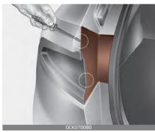
3. Loosen the lower light assembly retaining screw with a cross-tip screwdriver or spanner.
