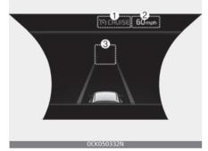
You can see the status of the Smart Cruise Control operation in the Driving Assist view on the cluster. Refer to "Instrument cluster" on page 4– 68.
