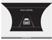
• Navigation-based Smart Cruise Control is not able to slow down your vehicle to a safe speed.
