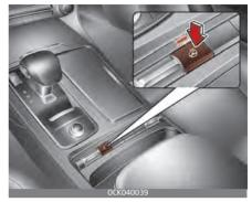
With the ENGINE START/STOP Button in the ON position, pressing the heated steering wheel button warms the steering wheel. The indicator on the button will illuminate.
