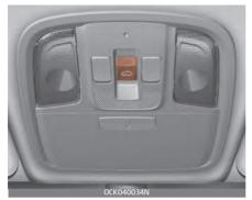
You can operate the sunroof with the sunroof switch in the ignition ON position.
