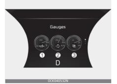
This mode displays Oil temperature (1), Torque gauge (2), Turbo boost gauge (3).
