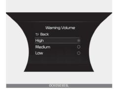
With the ENGINE START/STOP button in the ON position, select 'Driver Assistance  $\rightarrow$  Warning Volume' from the "User Settings (LCD display) or Setup  $\rightarrow$  Vehicle (Infotainment System screen)" to change the Warning Volume to 'High', 'Medium', 'Low' for Lane Keeping Assist.
