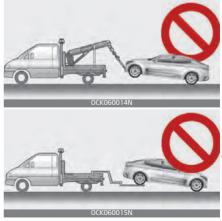
• Do not tow the vehicle backwards with the rear wheels on the
