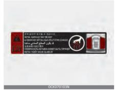
Do not touch metal surfaces in the trunk under the compartment cover while the engine is operating or hot. Doing so could result in serious personal injury.
