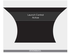
If both the brakes and accelerater pedals were applied and the driver removes his foot only from the accelerater pedal, Launch Control will be automatically deactivated. Or, if the vehicle does not start after 4 seconds with a driver's feet on both brake and accelerate pedals, Launch Control will automatically deactivated as well.
