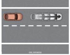
If the vehicle in front abruptly departures, Leading Vehicle Departure Alert may not operate properly.
