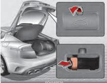
Your vehicle is equipped with the emergency liftgate safety release lever located on the bottom of the liftgate. When someone is inadvertently locked in the luggage compartment, the liftgate can be opened by doing as follows:
