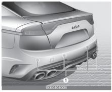
Refer to the picture above for the detailed location of the rear ultrasonic sensors (1).
