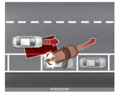
When changing lanes by detecting the lane ahead, if the function judges that there is a collision risk with an approaching vehicle in the blind spot, the function will help avoid collision by applying the differential brake.
