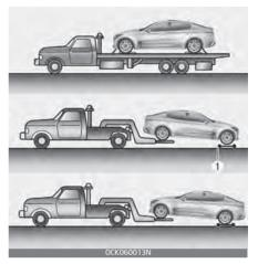
If emergency towing is necessary, we recommend having it done by an authorized Kia dealer or a commercial tow-truck service. Proper lifting and towing procedures are necessary to prevent damage to the vehicle. The use of wheel dollies(1) or flatbed is recommended.
