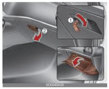
The glove box can be locked and unlocked with a master key (1). (if equipped)
