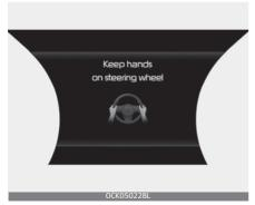
If the driver takes their hands off the steering wheel for several seconds, the 'Keep hands on steering wheel' warning message will appear on the cluster, and an audible warning will sound in stages.
