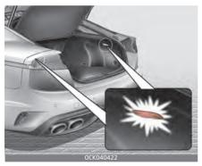
The liftgate room lamp comes on when the liftgate is opened.
