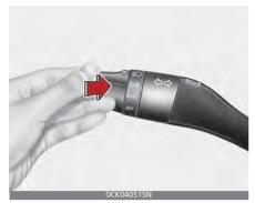
To turn on the high beam headlamp, push the lever away from you when the headlight is on.
