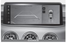
Surround View Monitor can assist in parking by allowing the driver to see around the vehicle.
