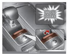
1. Depress the brake pedal. 2. Pull up the EPB switch.
