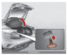
If the fuel filler door does not open using the fuel filler door opener button, you can open it manually by pulling the handle outward slightly.
