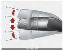
The ENGINE START/STOP button must be on for the turn signals to function. To turn on the turn signals, move the lever up or down (A). The green arrow indicators on the instrument panel indicate which turn signal is operating. They will self-cancel after a turn is completed. If the indicator continues to flash after a turn, manually return the lever to the OFF position.
