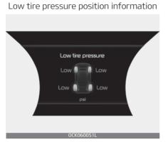
When the tire pressure monitoring system warning indicators are illuminated, one or more of your tires is significantly under-inflated.
