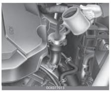
\* (For Smartstream G2.5 FR T-GDi) After removing the engine cover, fill up the engine oil.
