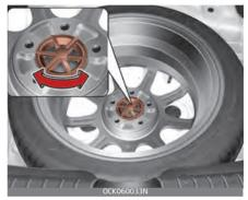
Turn the tire hold-down wing bolt counterclockwise.
