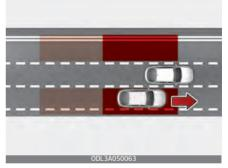
Blind-Spot Collision-Avoidance Assist help detects and informs the driver that a vehicle is in the blind spot.
