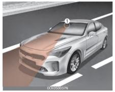
The front view camera (1) is used as a detecting sensor to detect ambient light and brightness while driving. Refer to the picture above for the detailed location of the detecting sensor.
