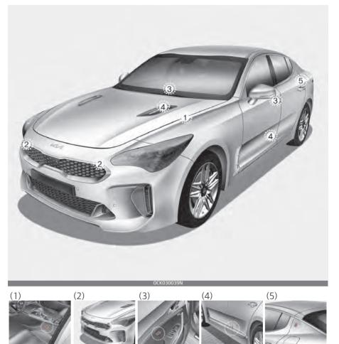
1. SRS control module/ Rollover sensor
