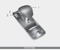
When you move the shift lever (1), depress the brake pedal while pressing the UNLOCK button (2).
