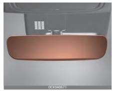
The electric rearview mirror automatically controls the glare from the headlights of the vehicles behind you in nighttime or low light driving conditions. The sensor mounted in the mirror senses the light level around the vehicle, and automatically controls the headlight glare from the vehicles behind you.
