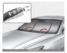
For your convenience, move the windshield wiper blades to the service position as follows; After turning off the engine, move the wiper switch to the single wiping (MIST) position within 20 seconds and hold the switch more than 2 seconds until the wiper blade is in the fully up position.
