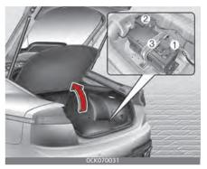
The battery is in the trunk under the compartment cover.
