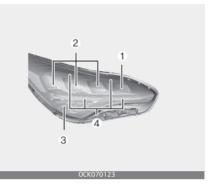
If the High beam lamp (1), Low beam lamp (2), High beam assist lamp (3), Front turn signal lamp (4), Day time running lamp/Position lamp (5) or Side maker (6) does not operate, have the vehicle checked by an authorized Kia dealer.
