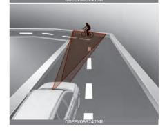
Forward Collision–Avoidance Assist may detect a vehicle or pedestrian in the next lane or outside the lane when driving on a curved road. If this occurs, the unnecessarily alarm the driver and apply the brake. Always check the traffic conditions around the vehicle.
