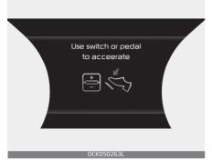
In traffic, your vehicle will stop if the vehicle ahead of you stops. Also, if the vehicle ahead of you starts moving, your vehicle will start as well. In addition, after the vehicle has stopped and a certain time have passed, the 'Use switch or pedal to accelerate' message will appear on the cluster. Depress the acceleratorpedal or push the + switch, - switch or || ) switch to start driving.
