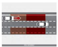
Blind-Spot Collision-Avoidance Assist help detects and informs the driver that a vehicle is approaching at high speed from the blind spot area.
