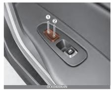
Operate by pressing the central door lock switch.
