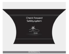
When Forward Collision-Avoidance Assist is not working properly, the 'Check Forward Safety system' warning message will appear, and the sign and warning lights will illuminate on the cluster. In this case, have the vehicle inspected by an authorized Kia dealer.
