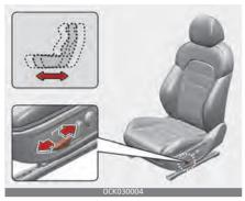
Push the control switch forward or backward to move the seat to the desired position. Release the switch once the seat reaches the desired position.
