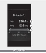
• Fuel efficiency is calculated after the vehicle has run for more than 0.2 miles (300 meters).
