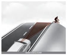
Forward Collision–Avoidance Assist may not detect other vehicle, pedestrian or cyclist in front while driving uphill or downhill and this may result in no warning, braking assist or steering assist when necessary.
