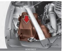
The air filter must be replaced when necessary, and should not be washed.
