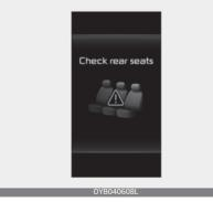
You can activate or deactivate the Rear Occupant Alert by selecting 'User Settings (LCD display) or Setup  $\rightarrow$  Vehicle (Infotainment System screen)  $\rightarrow$  Convenience  $\rightarrow$  Rear Occupant Alert'.
