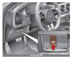
With the ENGINE START/STOP button in the ON position, press and hold the Lane Safety button located on the instrument panel to turn on Lane Keeping Assist. The white indicator light ( ) will illuminate on the cluster. Press and hold the button again to turn off the function.
