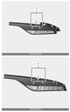
If the stop and tail lamp (LED) (1,2), does not operate, have the vehicle checked by an authorized Kia dealer.
