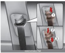
You can adjust the height of the shoulder belt anchor to one of 4 positions for maximum comfort and safety.
