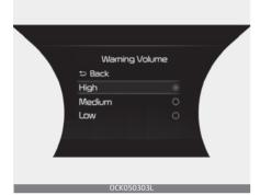
With the ENGINE START/STOP button in the ON position, select 'Driver Assistance  $\rightarrow$  Warning Volume' from the "User Settings (LCD display) or Setup  $\rightarrow$  Vehicle (Infotainment System screen)" to change the warning volume to 'High', 'Medium', 'Low' for Highway Driving Assist.
