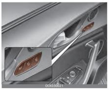
Driving Position Memory System is the facility that enables driver's seat, steering wheel, outside rear view mirrors and head-up display (HUD) to be controlled with a simple button operation, which allows a driver to recall memorized driving positions to suit your preferences.
