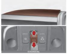
Press the sunroof switch upward and glass tilt open (if the blind is closed, blind slide open first).
