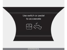
When Highway Driving Assist is operating, your vehicle will stop if the vehicle ahead of you stops. Also, if the vehicle ahead of you starts moving within 30 seconds after the stop, your vehicle will start as well. In addition, after the vehicle has stopped and 30 seconds have passed, the 'Use switch or pedal to accelerate' message will appear on the cluster. Depress the accelerator pedal or push the + switch, - switch or (|| )) switch to start driving.
