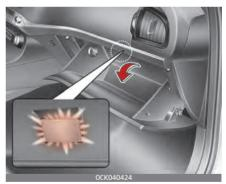
The glove box lamp comes on when the glove box is opened.
