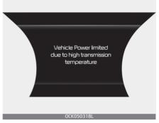
This message is displayed when the transmission oil temperature is high. Drive at steady speed or stop the vehicle at a safe place with the engine on. When the oil temperature returns to normal, the message will disappear.
