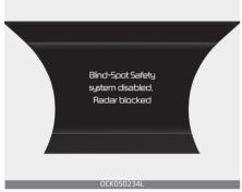
When the rear bumper around the rear corner radar or sensor is covered with foreign material, such as snow or rain, or installing a trailer or carrier, it can reduce the detecting performance and temporarily limit or disable Blind–Spot Safety system.
