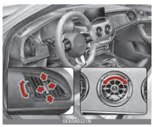
The outlet vents can be opened or closed separately using the thumb-wheel.
