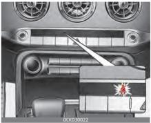
As a reminder to the front passenger, the front passenger's seat belt warning lights will illuminate for approximately 6 seconds each time you turn the Engine start/stop button in ON regardless of belt fastening.
