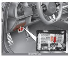
Always set the fuse switch to the ON position before using the vehicle.
