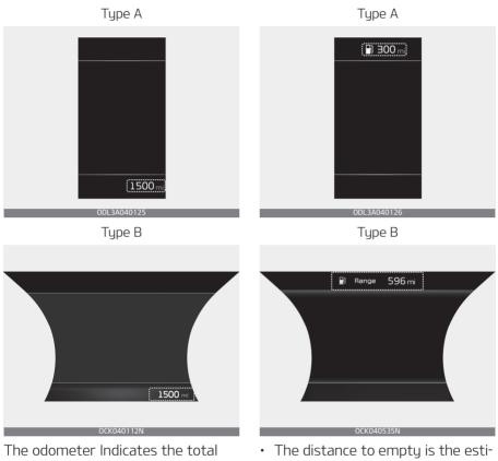
The odometer Indicates the total distance that the vehicle has been driven and should be used to determine when periodic maintenance should be performed.
