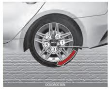
Position the wrench as shown in the drawing and tighten the wheel nuts. Be sure the socket is seated completely over the nut. Do not stand
