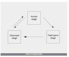
This system is designed to provide protection from unauthorized entry into the vehicle. This system is operated in three stages: the first is the "Armed" stage, the second is the "Theft-alarm" stage, and the third is the "Disarmed" stage. If triggered, the system provides an audible alarm with blinking of the hazard warning lights.
