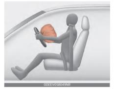
A fully inflated air bag, in combination with a properly worn seat belt, slows the driver's or the passenger's forward motion, reducing the risk of head and chest injury. 3
