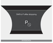
The warning message appears on the LCD display, when the brake
