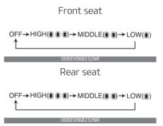
• The seat warmer defaults to the OFF position whenever the ENGINE START/STOP button is turned on.
