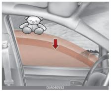
If the upward movement of the window is blocked by an object or part of the body, the window will detect the resistance and will stop upward movement. The window will then lower approximately 11.8 in. (30 cm) to allow the object to be cleared.
