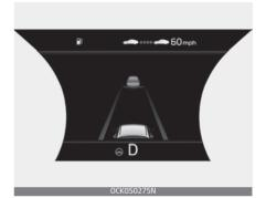
If the vehicle ahead or both lane markings are detected and your vehicle speed is below 120 mph (200 km/h), the green () indicator light will illuminate on the cluster, and the function will help the vehicle stay in lane by controlling the steering wheel.
