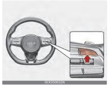
Press the Driving Assist S button to turn on the function. The speed will be set to the current speed on the cluster.
