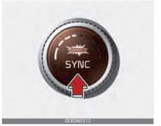
• Press the "SYNC" button to adjust the driver and passenger side temperature equally.
