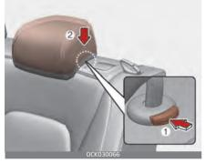
4. Pull on the seatback folding lever(1), then fold the seat toward the front of the vehicle.
