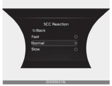
The sensitivity of vehicle speed when following the front vehicle to maintain the set distance can be adjusted. Go to the "User Settings (LCD display) or Setup  $\rightarrow$  Vehicle (Infotainment System screen)  $\rightarrow$ Driver Assistance  $\rightarrow$  SCC Reaction  $\rightarrow$ Fast/Normal/Slow". You may select one of the three stages you prefer.
