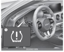
2. Low tire pressure position telltale (Shown on the LCD display)
