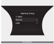
With the ENGINE START/STOP button in the ON position, select 'Driver Assistance  $\rightarrow$  Warning Timing' from the "User Settings (LCD display) or Setup  $\rightarrow$  Vehicle (Infotainment System screen)" menu to change the initial warning activation time for Forward Collision-Avoidance Assist.
