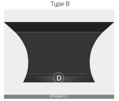
This indicator displays which automatic transmission shift lever is selected.
