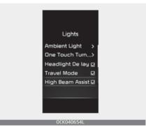
By selecting as 'User Settings (LCD display) or Setup  $\rightarrow$  Vehicle (Infotainment System screen)  $\rightarrow$  Lights  $\rightarrow$  High Beam Assist' on the cluster LCD display or the Infotainment System screen at engine ON, you may select or release the function. The settings will remain even if engine OFF and ON.
