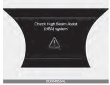
When High Beam Assist is not working properly, the 'Check High Beam Assist (HBA) system' warning message will appear on the cluster (turns off after a certain time) and ( ) warning light will illuminate.
