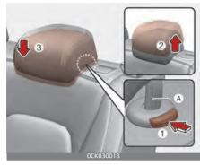
To remove the headrest, raise it as far as it can go then press the release button (1) while pulling the headrest upward (2).
