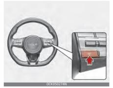
With the ENGINE START/STOP button in the ON position, press the Lane Driving Assist button A located on the steering wheel to turn on Lane Following Assist. The white or green () indicator light will illuminate on the cluster.
