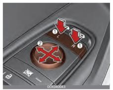
The electric remote control mirror switch allows you to adjust the position of the left and right outside rearview mirrors. To adjust the position of either mirror, press the R or L button (1) to select the right side mirror or the left side mirror, then press a corresponding point ( $\blacktriangle$ ) (2) on the mirror adjustment control to position the selected mirror up, down, left or right.
