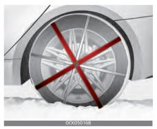
Since the sidewalls on some radial tires are thinner than other types of tires, they may be damaged by mounting certain types of tire chains on them. Therefore, the use of snow tires is recommended instead of tire chains. Do not mount tire chains on vehicles equipped with aluminum wheels; if unavoidable, use AutoSock (fabric snow chain). Install the tire chain after reviewing the instructions provided with the tire chains.
