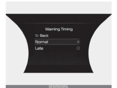
With the ENGINE START/STOP button in the ON position, select 'Driver Assistance  $\rightarrow$  Warning Timing' from the "User Settings (LCD display) or Setup  $\rightarrow$  Vehicle (Infotainment System screen)" menu to change the initial warning activation time for Rear Cross-Traffic Safety system.
