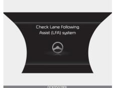
When Lane Following Assist is not working properly, the 'Check Lane Following Assist (LFA) system' warning message will appear on the cluster (turns off after a certain time) and ( ) warning light will illuminate.
