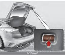
The driver may set the height of a fully opened liftgate by following the below instruction.
