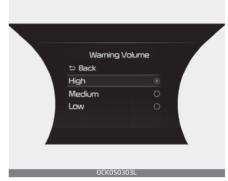
With the ENGINE START/STOP button in the ON position, select 'Driver Assistance  $\rightarrow$  Warning Volume' from the "User Settings (LCD display) or Setup  $\rightarrow$  Vehicle (Infotainment System screen)" to change the Warning Volume to 'High', 'Medium', 'Low' for Blind-Spot Safety system.
