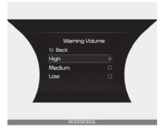
With the ENGINESTART/STOP button in the ON position, select 'Driver Assistance  $\rightarrow$  Warning Volume' from the "User Settings (LCD display) or Setup  $\rightarrow$  Vehicle (Infotainment System screen)" menu to change the Warning Volume to 'High', 'Medium', 'Low' for Smart Cruise Control.
