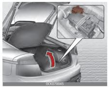
Inside the fuse/relay panel covers, you can find the fuse/relay label describing fuse/relay name and capacity.
