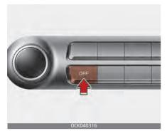
Press the front blower OFF button to turn off the front air climate control system. However, you can still operate the mode and air intake buttons as long as the ENGINE START/STOP button is in the ON position.
