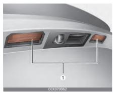
If the license plate lamp (LED) (1) does not operate, have the vehicle checked by an authorized Kia dealer.
