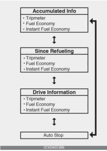
To change the trip mode, scroll the toggle the switch  $(\frown / \checkmark)$  on the steering wheel.
