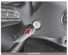
When the stop lamp fuse is blown, you can't start the engine normally. Replace the fuse with a new one. If it is not possible, you can start the engine by pressing the ENGINE START/STOP button for 10 seconds while it is in the ACC position. The engine can start without depressing the brake pedal. But for your safety always depress the brake pedal before starting the engine.
