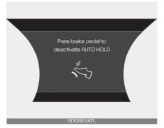
If you do not apply the brake pedal when you release the Auto Hold by pressing the [AUTO HOLD] switch, a warning will sound and a message will appear.
