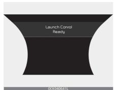
To start a vehicle, with your right foot pressing the accelerator pedal down fully, remove your left foot from the brake. (within 4 seconds) (Launch Control Active (2) Status Display on Cluster Screen)
