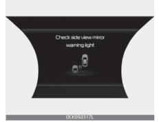
When the side view mirror (outside mirror) warning light is not working properly, the 'Check side view mirror warning light' warning message will appear on the cluster. In this case, have your vehicle inspected by an authorized Kia dealer.
