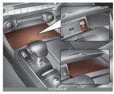
A wireless smart phone charging system is located in front of the center console.
