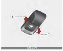
To open or close a window, press down or pull up the front portion of the corresponding switch to the first detent position (5).
