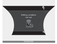
The warning message appears on the LCD display, when engine RPM is too high, or when driving speed is too fast to shift the gear. We recommend you decrease your RPM level or slow down before shifting the gear.
