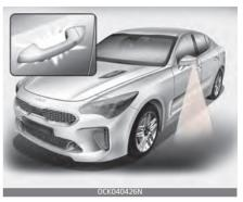
When all the doors (and liftgate) are locked and closed, the pocket lamp and puddle lamp, room lamp will come on for about 15 seconds if any of the below is performed.
