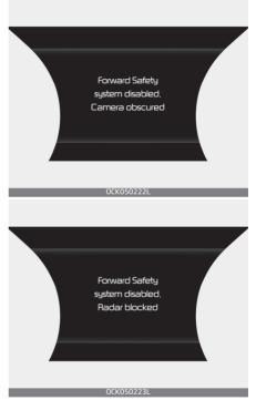
When the front windshield where the front view camera is located, front radar cover or sensor is covered with foreign material such as snow or rain, it can reduce the detecting performance and temporarily limit or disable Forward Collision-Avoidance Assist. If this occurs the 'Forward Safety system disabled. Radar blocked' warning message, and the S and M warning lights will illuminate on the cluster.
