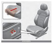
1. Push the front part of control switch to move the seat cushion to the desired length. 2. Release the switch once the seat cushion reaches the desired length.
