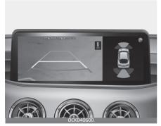
You can change Rear View Monitor settings by pressing the setup icon (◊) on the screen while the function is operating, or select 'Setup → Vehicle (Infotainment)
