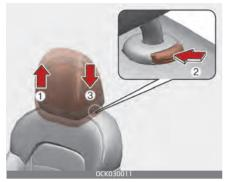
To raise the headrest, pull it up to the desired position (1). To lower the headrest, push and hold the release button (2) and lower the headrest to the desired position (3).
