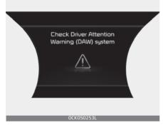
When Driver Attention Warning is not working properly, the 'Check Driver Attention Warning (DAW) system' warning message will appear on the cluster (turns off after a certain time) and ( ) warning light will illuminate. In this case, have your vehicle inspected by an authorized Kia dealer.
