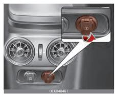
The USB charger is designed to recharge devices using a USB cable.
