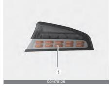
If the rear turn signal lamp (LED) (1), does not operate, have the vehicle checked by an authorized Kia dealer.
