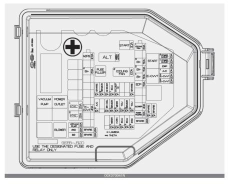
Engine compartment fuse panel
