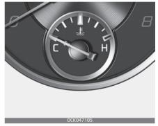
This gauge indicates the temperature of the engine coolant when the ENGINE START/STOP button is ON.
