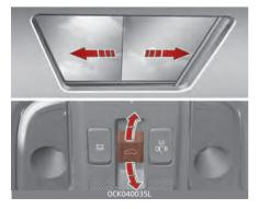
Press the sunroof switch backward and glass slide open(if the blind is closed, blind slide open first).
