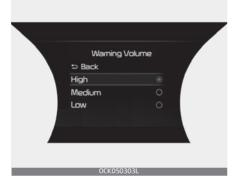
With the ENGINESTART/STOP button in the ON position, select 'Driver Assistance  $\rightarrow$  Warning Volume' from the "User Settings (LCD display) or Setup  $\rightarrow$  Vehicle (Infotainment System screen)" menu to change the Warning Volume to 'High', 'Medium', 'Low' for Rear Cross-Traffic Safety system.
