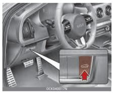
Press the power liftgate close button for approximately one second when the liftgate is opened. The liftgate will close and lock automatically.
