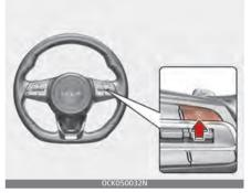
Press the Driving Assist 💫 button to turn Smart Cruise Control off.
