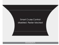
When the front radar cover or sensor is covered with snow, rain, or foreign matters, it can reduce the detecting performance and temporarily limit or disable Smart Cruise Control.
