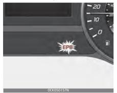
This warning light illuminates if the ENGINE START/STOP button is changed to the ON position and goes off in approximately 3 seconds if the system is operating normally.
