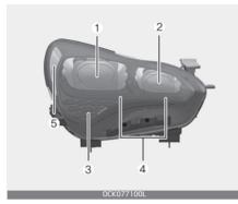
If the Low/High beam lamp(1), Low/ High beam assist lamp (2), Front turn signal lamp (3), Day time running lamp/Position lamp (4) or Side marker (5) does not operate, have the vehicle checked by an authorized Kia dealer.
