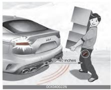
If you are positioned in the detecting area (20 ~ 40 inches (50 ~100 cm) behind the vehicle) carrying a smart key, the hazard warning lights will blink and the chime will sound for about 3 seconds to alert you the smart key has been detected and the liftgate will open.
