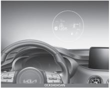
The Head Up Display is a transparent display which projects some information of the instrument cluster and navigation on the windshield alass.
