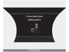
When Blind-Spot Safety system is not working properly, the 'Check Blind-Spot Safety system' warning message will appear (turns off after a certain time), and ( ) warning light will illuminate on the cluster. In this case, have your vehicle inspected by an authorized Kia dealer.
