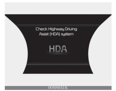
When Highway Driving Assist is not working properly, the 'Check Highway Driving Assist (HDA) system' warning message will appear, and the ( ) warning light will illuminate on the cluster.
