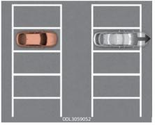
If a vehicle parked in front drives away from you, Leading Vehicle Departure Alert may warn you that the parked vehicle is driving away. • When driving at a tollgate or intersection, etc.
