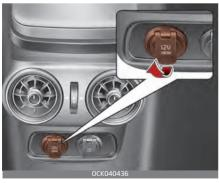
The power outlet is designed to provide power for mobile devices.
