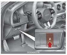
The fuel filler door must be opened from inside the vehicle by pressing the fuel filler door opener button.
