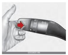
To flash the headlights, pull the lever towards you. It will return to the normal (low beam) position when released. The headlight switch does not need to be on to use this flashing feature.
