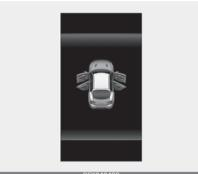
• This warning is displayed indicating which door, or the hood, or the liftgate is open.
