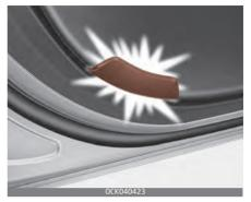
The door courtesy lamp comes ON when the door is opened to assist entering or exiting the vehicle. It also serves as a warning to passing vehicles that the vehicle door is open.
