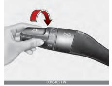
When the light switch is in the parking light position, the tail, license and parking lights will turn ON.
