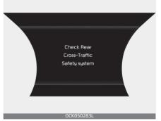
When Rear Cross-Traffic Safety system is not working properly, the 'Check Rear Cross-Traffic Safety system' warning message will appear on the cluster, and the function will turn off automatically or the function will be limited. In this case, have your vehicle inspected by an authorized Kia dealer.
