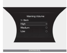
With the ENGINE START/STOP button in the ON position, select 'Driver Assistance  $\rightarrow$  Warning Volume' from the "User Settings (LCD display) or Setup  $\rightarrow$  Vehicle (Infotainment System screen)" menu to change the Warning Volume to 'High', 'Medium', 'Low' for Forward Collision-Avoidance Assist.
