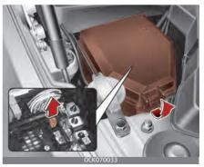
Check the removed fuse; replace it if it is blown.
