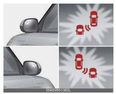
If a vehicle is detected within the boundary of the function, a warning light will illuminate on the outer side view mirror and the Head-Up Display (if equipped).
