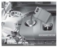
Use a funnel to help prevent oil from being spilled on engine components. Use only the specified engine oil. "Recommended lubricants and capacities" on page 8-7
