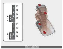
Depress the brake pedal and the lock release button when shifting.
