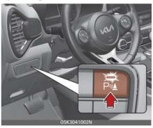
This function activates when the Parking Safety button is pressed with the ignition switch or ENGINE START/STOP button ON.
