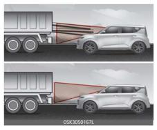
When the vehicle in front has heavy loading extended rearward, or when the vehicle in front has higher
