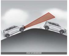
During uphill or downhill driving, Smart Cruise Control may not immediately detect a moving vehicle in your lane, and may cause your vehicle to accelerate to the set speed.
