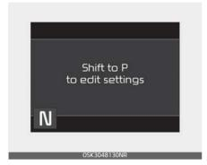
For your safety, change the User Settings after parking the vehicle, applying the parking brake and moving the shift lever to P (Park). Features of your vehicle LCD display
