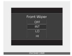
This indicator displays which wiper speed is selected using the wiper control.
