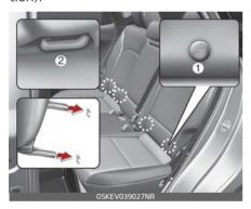
1. Lower Anchor position indicator2. Lower Anchor
