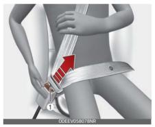
The seat belt is released by pressing the release button (1) on the locking buckle.
