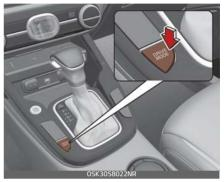
The mode changes whenever the DRIVE MODE button is pressed.
