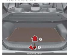
3. Pull the luggage board hinge to the end of upper side sliding slot and it will fall down lower to increase cargo space.
