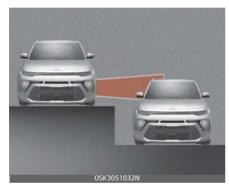
Blind-Spot Collision Warning may not operate properly when driving where the heights of the lanes are different.
