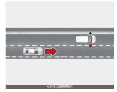
Blind-Spot Collision Warning will warn you when it detects a vehicle is approaching in an adjacent lane at a high rate of speed. If the driver activates the turn signal when the system detects an oncoming vehicle, the system sounds an audible warning.
