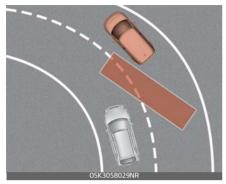
Blind-Spot Collision Warning may not operate properly when driving on a curved road. In certain instances, the function may not detect the vehicle in the next lane.
