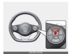
When Smart Cruise Control is not needed, press the [CRUISE] switch and deactivate the function.
