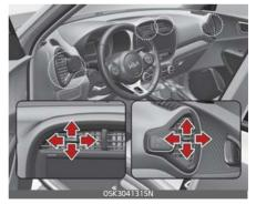
Also, you can adjust the direction of air delivery from these vents using the vent control lever as shown.
