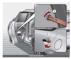
To lock the child safety lock, insert a key (or screwdriver) into the hole and turn it to the lock position.
