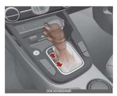
SPORT mode manages the driving dynamics by automatically adjusting the steering effort, and the engine and transmission control logic for enhanced driver performance.
