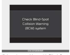
If there is a problem with Blind-Spot Collision Warning, a warning message will appear and the light on the switch will turn off. The function will turn off automatically. Rear Cross-Traffic Collision Warning and Rear Cross-Traffic Collision-Avoidance Assist will not operate also if Blind-Spot Collision Warning turns off due to malfunction. Have your vehicle inspected by an authorized Kia dealer
