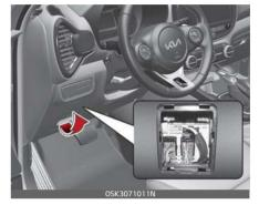
3. Pull the suspected fuse straight out. Use the removal tool provided on the engine fuse panel cover.
