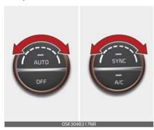
The temperature will increase to the maximum (82 °F (28 °C)) by turning the knob to the extreme right.
