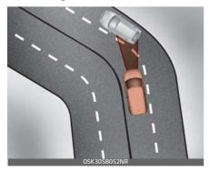
Your vehicle speed can be reduced due to a vehicle in the adjacent lane. Adjust your vehicle speed by
