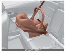
A rear-facing child seat provides restraint with the seating surface against the back of the child. The harness system holds the child in place, and in an accident, acts to
