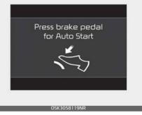
If you move the transmission lever from N to D (manual mode) or R without depressing the brake pedal after stopping engine automatically, the engine does not restart automatically and a warning chime alarms. When this happens, press the brake pedal for auto start.
