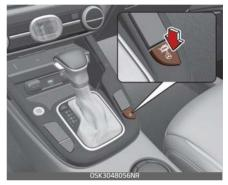
To turn the heated steering wheel off, press the button once again.
