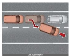
When vehicles are at a standstill and the vehicle in front of you changes to the next lane, be careful when your vehicle starts to move because it may not immediately recognize the stopped vehicle in front of you.
