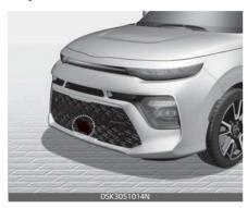
The front radar detects the distance to the vehicle ahead.
