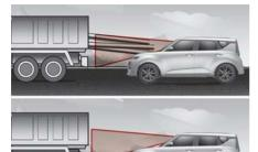
When the vehicle in front has heavy loading extended rearward, or when the vehicle in front has higher ground clearance, it may induce a hazardous situation. Always pay attention to road and driving conditions, while driving and, if necessary, depress the brake pedal to reduce your driving speed in order to maintain distance.
