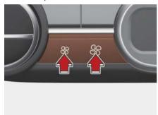
To turn the fan speed control off, press the front blower OFF button.
