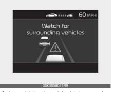
If the vehicle ahead (vehicle speed: less than 20 mph (30 km/h)) moves to the next lane, the warning chime will sound and a message will appear. Adjust your vehicle speed for vehicles or objects that can suddenly appear in front of you by
