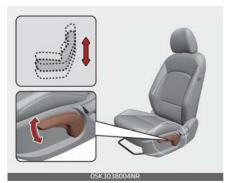
To change the height of the seat cushion, push the lever upwards or downwards.
