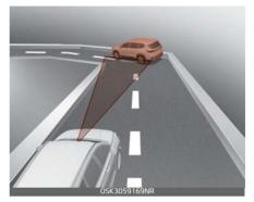
Forward Collision–Avoidance Assist may recognize a vehicle in the next lane or outside the lane when driving on a curved road. If this occurs, the function may unnecessarily alarm the driver and apply the brake.
