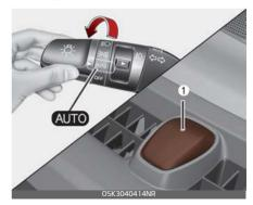
When the light switch is in the AUTO light position, the taillights and headlights will turn ON or OFF auto-
