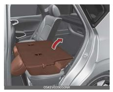
1. To use the rear seat, lift and pull the seatback backward. Pull the seatback firmly until it clicks into place. Make sure the seatback is locked in place. When you return the seatback to its upright position, always be sure it has locked into position by pushing on the top of the seatback.
