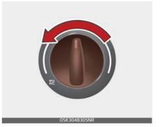
In this mode, the air conditioning and the recirculated air position will be selected automatically.
