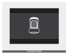
If the driver turns off the engine when the sunroof is not fully closed, the warning chime will sound for several seconds and the sunroof open warning will appear on the cluster LCD display.
