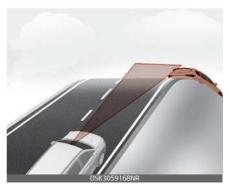
The performance of Forward Collision–Avoidance Assist may be decreased while driving upward or downward on a slope.
