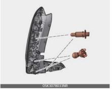
Remove the bulb from the socket by pressing it in and rotating it counterclockwise until the tabs on
