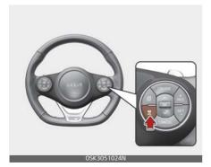
The vehicle distance will automatically activate when Smart Cruise Control is on.
