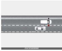
The blind spot detection range varies relative to vehicle speed. Note that if your vehicle is traveling much faster than the vehicles around you, the warning will not occur.
