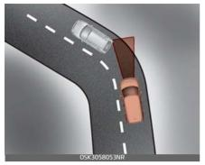
On curves, Smart Cruise Control may not immediately detect a moving vehicle in your lane, and then your vehicle could accelerate to the set speed. Also, the vehicle speed will rapidly decrease when the vehicle ahead is recognized suddenly.
