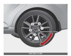
18.After changing wheels, have an authorized Kia dealer tighten the wheel nuts to their proper torque as soon as possible.
