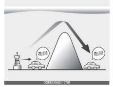
AM broadcasts can be received at greater distances than FM broadcasts. This is because AM radio waves are transmitted at low frequencies. These long distance, low frequency radio waves can follow the curvature of the earth rather than traveling straight. In addition,
