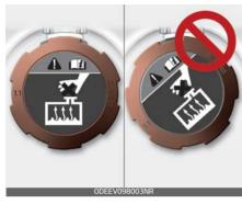
2. Maker sure that the tiny protrusions inside the coolant cap are securely interlocked.
