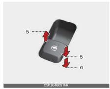
Pressing the power window switch momentarily to the second detent position (6) completely lowers the window even when the switch is released. To stop the window at the desired position while the window is in operation, pull up the switch briefly to the opposite direction of the window movement.
