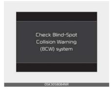
If there is a problem with Blind-Spot Collision Warning, a warning message will appear and the light on the switch will turn off. The function will turn off automatically. Have your vehicle inspected by an authorized Kia dealer
