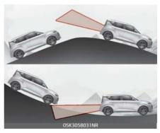
Blind–Spot Collision Warning may not operate properly when driving on a slope. In certain instances the function may not detect the vehicle in the next lane.
