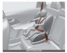
A forward-facing child seat provides restraint for the child's body with a harness. Keep children in a forwardfacing child seat with a harness until they reach the top height or weight limit allowed by your child restraint's manufacturer. Once your child outgrows the forward- facing child restraint, your child is ready for a booster seat.
