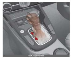
Whether the vehicle is stationary or in motion, manual mode is selected by pushing the shift lever from the
