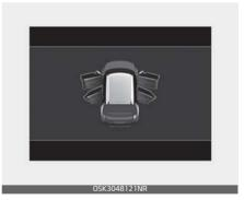
This warning is displayed if any door or the hood or the liftgate is left open. The warning will indicate which door is open in the display.
