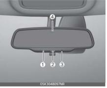
The electric rearview mirror automatically controls the glare from the headlights of the vehicles behind you in nighttime or low light driving conditions. The sensor (4) mounted in the mirror senses the light level around the vehicle, and automatically controls the headlight glare from the vehicles behind you.
