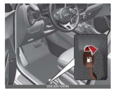
If the fuel filler door does not open because ice has formed around it. tap lightly or push on the door to break the ice and release the door. Do not pry on the door. If necessary, spray around the door with an approved de-icer fluid (do not use radiator anti-freeze) or move the vehicle to a warm place and allow the ice to melt.
