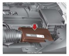
You can clean the filter when inspecting the air cleaner element. Clean the filter by using compressed air.
