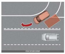
Blind-Spot Collision Warning may not operate properly when driving where the road is merging/dividing. In certain instances, the function may not detect the vehicle in the next lane.
