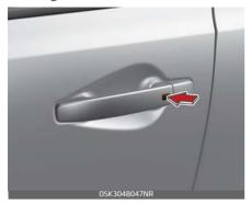
Pressing the button of the front outside door handles with all doors closed and any door unlocked, locks all the doors (and hood, liftgate). The hazard warning lights will blink once to indicate that all doors are locked. The button will only operate when the smart key is within 28~40 inches (0.7~1 m) from the outside door handle. If you want to make sure that a door has locked or not, you should check the door lock button inside the vehicle or pull the outside door handle.
