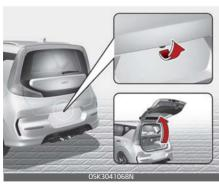
Only the liftgate is unlocked if the liftgate unlock button on the transmitter or smart key is pressed for approximately 1 second.
