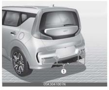
The sensing range and objects detectable by the sensors (1) are limited. Whenever moving pay as
