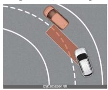
Blind-Spot Collision Warning may not operate properly when driving on a curved road. In certain instances, the function may recognize a vehicle in the same lane.
