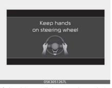
If the driver still does not have their hands on the steering wheel after several seconds, the function will only warn the driver when the driver crosses the lane lines. In this scenario, the function does not provide any steering inputs into the vehicle for you. Accordingly, you must take the necessary steps to maintain control of the vehicle and keep it within the lanes.
