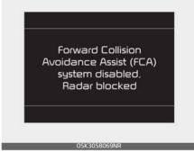
In this case, a warning message ("Forward Collision–Avoidance Assist (FCA) system disabled. Radar blocked") will appear to notify the driver. Remove the foreign substances to allow Forward Collision– Avoidance Assist to function normally.
