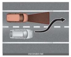
When a vehicle changes lanes in front of you, Forward Collision– Avoidance Assist may not immediately detect the vehicle, especially if the vehicle changes lanes abruptly. In this case, you must maintain a safe braking distance, and if necessary, depress the brake pedal to reduce your driving speed in order to maintain a safe distance.
