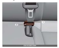
If the center seat belt is not in use, always lock the latch plate into the buckle as above illustration
