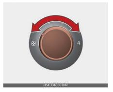
Setting the fan speed control knob to the "0" position turns off the fan.
