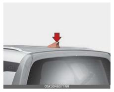
The shark fin antenna will receive the transmit data.
