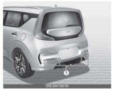
Reverse Parking Distance Warning is a supplemental function and it is not intended to nor does it replace the need for extreme care and attention of the driver. The sensing range and objects detectable by the back sensors (1) are limited. Whenever backing-up, pay as much attention to what is behind you as you would in a vehicle without Reverse Parking Distance Warning.
