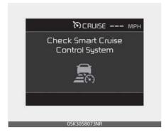
The message will appear when the vehicle distance control function is not functioning normally.
