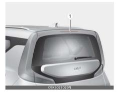
The LED lamps cannot be replaced as a single component because it is an integrated unit. The LED lamps has to be replaced with the unit.
