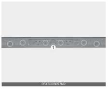
4. Pull out the bulb-socket from the high mounted stop lamp assembly using the driver.
