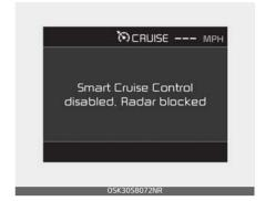
When the sensor lens cover is blocked with dirt, snow, or debris, Smart Cruise Control operation may stop temporarily. If this occurs, a warning message will appear on the LCD display. Remove any dirt, snow, or debris and clean the radar sensor lens cover before operating Smart Cruise Control.
