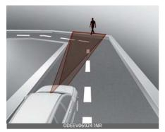
Forward Collision–Avoidance Assist may recognize a vehicle or pedestrian or cyclist in the next lane or outside the lane when driving on a curved road.
