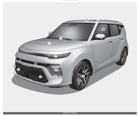
\* The actual shape may differ from the illustration. 1. Hood 4-31 4-92 2. Head lamp (Features of your vehicle) Head lamp (Maintenance) 7-67 3. Front fog lamp (Features of your vehicle) 4-95 Front fog lamp (Maintenance) 7-71 7-37 4. Wheel and tire (Maintenance) Wheel and tire (Specification) 8-5 5. Outside rearview mirror 4-46 4-36 6. Sunroof 7. Front windshield wiper blades (Features of your vehicle) 4-99
