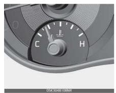
This gauge indicates the temperature of the engine coolant when the ignition switch or ENGINE START/
