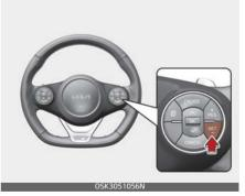
3. Push the SET- button, and release it at the desired speed. The cruise set indicator light will illuminate. Release the accelerator pedal at the same time. The
