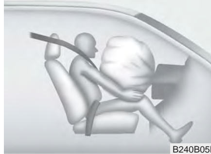
Passenger's front air bag
