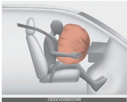
Passenger's front air bag
