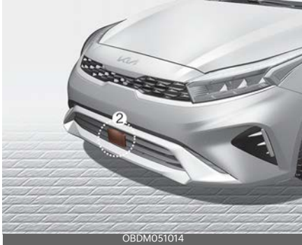
[1]: Front view camera, [2]: Front radar Refer to the picture above for the detailed location of the detecting sensors.
