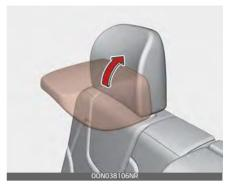
The headrest will fold down automatically when folding the seatback.
