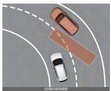
Blind-Spot Collision Warning and Blind-Spot Collision-Avoidance Assist may not operate properly when driving on a curved road. In certain instances the system may not detect the vehicle in the next lane.
