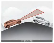
During uphill or downhill driving, Smart Cruise Control may not immediately detect a moving vehicle in your lane, and may cause your vehicle to accelerate to the set speed.
