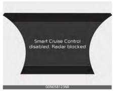
When the sensor lens cover is coverd with dirt, snow, or debris, Smart Cruise Control operation may stop temporarily. If this occurs, a warning message will appear on the LCD display. Remove any dirt, snow, or debris and clean the radar sensor lens cover before operating Smart Cruise Control.
