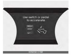
While Smart Cruise Control is in operation, your vehicle stops behind the vehicle in front when it stops. The message is displayed on the cluster within 3 seconds after the stop and the system will be in the standby position.
