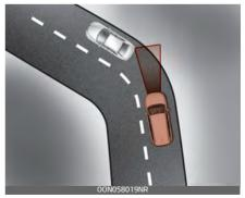
The Smart Cruise Control function may not detect a moving vehicle in
