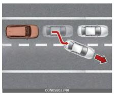
When driving in stop-and-go traffic, and a stopped vehicle in front of you merges out of the lane, the system may not immediately detect the new vehicle that is now in front of you.
