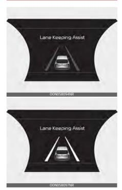
If the speed of the vehicle is over 40 mph (64 km/h) and Lane Keeping Assist detects lane markers, the color changes from gray to white.
