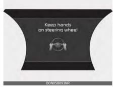
The hands-off warning appears when the system detects that the driver's hands are not on the steering wheel while Highway Driving Assist is in work.
