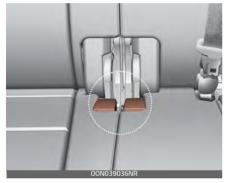
Route the seat belt webbing through the rear seat belt guides. It will help keep the belts from being trapped behind or under the seats.
