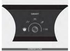
SMART mode: SMART mode automatically adjusts the driving mode (ECO ↔ COMFORT ↔ SPORT) in accordance with the driver's driving habits. 5
