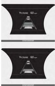
Your vehicle speed will slow down or speed up to maintain the selected distance. (A vehicle will appear in front of your vehicle in the LCD display only when there is an actual vehicle in front of you.)
