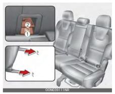
1. Lower Anchor position indicator 2. Lower Anchor
