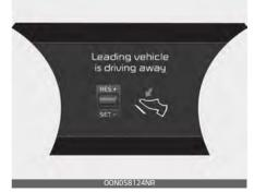
If the driver does not take action for a certain period of time after the vehicle in front departs, the message is displayed on the cluster. The vehicle departs automatically if the accelerator pedal is depressed or [RES +] or [SET –] switch is activated when there is a vehicle in front.
