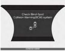
If there is a problem with Blind-Spot Collision Warning, a warning message will appear and the light on the switch will turn off. Rear Cross-Traffic Collision Warning and Rear Cross-Traffic Collision-Avoidance Assist will turn off automatically. Rear Cross-Traffic Collision Warning and Rear Cross-Traffic Collision-Avoidance Assist will not operate also if Blind-Spot Collision Warning turns off due to malfunction. Have your vehicle inspected by an authorized Kia dealer.
