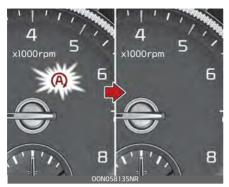
The engine will start and the green AUTO STOP indicator (A) on the instrument cluster will go out.
