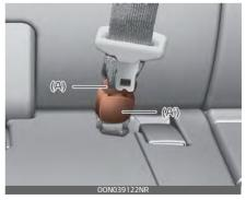
Pull out the tongue plate (B) from the pocket. Pull the tongue plate (B) and insert it into the buckle (B') until an audible "click" is heard, indicating the latch is locked.Make sure the belt is not twisted.
