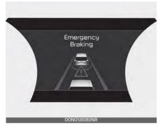
The warning message appears on the LCD display with the a warning chime.
