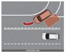
Blind-Spot Collision Warning and Blind-Spot Collision-Avoidance Assist may not operate properly when driving where the road is merging/dividing. In certain instances Blind-Spot Collision Warning and Blind-Spot Collision-Avoidance Assist may not detect the vehicle in the next lane. Always pay attention to road and driving conditions, while driving. Driving on a slope
