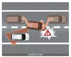
Blind-Spot Collision-Avoidance Assist may activate the Electronic Stability Control (ESC) in accordance with a colliding possibility with an approaching vehicle while changing lanes.
