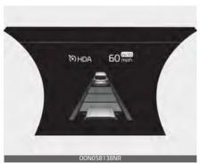
If Highway Driving Assist operating conditions are all met and setting speed matches with the legal highway speed limit, Highway Driving Assist will enter the automatic speed setting mode. (The set speed and the "AUTO" symbol will be displayed in green with an indicative sound)
