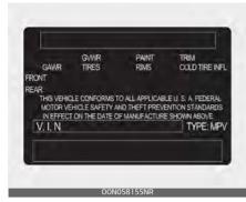
This label shows the maximum allowable weight of the fully loaded vehicle. This is called the GVWR (Gross Vehicle Weight Rating). The GVWR includes the weight of the vehicle, all occupants and cargo.
