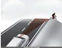
The performance of Forward Collision-Avoidance Assist may be decreased while driving upward or downward on a slope. The front view camera or front radar sensor recognition may not detect the vehicle, pedestrian or cyclist in front.
