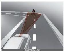
Forward Collision–Avoidance Assist may recognize a vehicle, pedestrian or cyclist in the next lane or outside the lane when driving on a curved road.
