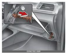
3. Remove the climate control air filter cover while pressing the lock on the upper side of the cover.
