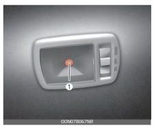
If the luggage lamp (LED) (1) does not operate, have the vehicle checked by an authorized Kia dealer. The LED lamps cannot be replaced as a single component because they are part of an integrated unit. The LED lamps have to be replaced with the unit.
