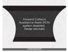
In this case, a warning message ("Forward Collision-Avoidance Assist (FCA) system disabled. Radar blocked") will appear to notify the driver.
