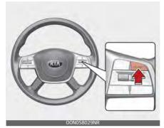
When Smart Cruise Control is not needed, press the [CRUISE] switch and deactivate the system.
