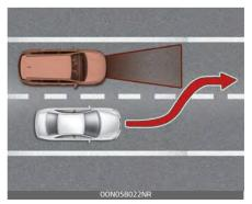
A vehicle which moves into your lane from an adjacent lane cannot be recognized by the sensor until it is in the sensor's detection range.
