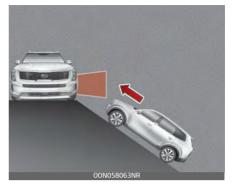
Rear Cross-Traffic Collision Warning and Rear Cross-Traffic Collision-Avoidance Assist may not operate properly when the vehicle is on/near a slope.
