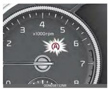
The engine will stop and the green AUTO STOP (A) indicator on the instrument cluster will illuminate.
