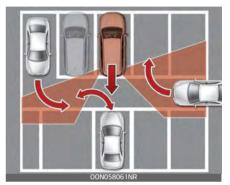
Rear Cross-Traffic Collision Warning and Rear Cross-Traffic Collision-Avoidance Assist may not operate properly when the vehicle is in a complex parking environment.
