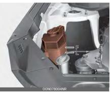
Do not remove the radiator cap when the engine and radiator are hot. Scalding hot coolant and steam may blow out under pressure which may result in serious injury.
