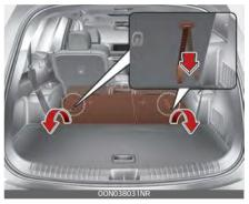
To use the rear seat, lift and pull the seatback backward. Pull the seatback firmly until it clicks into place. Make sure the seatback is locked in place. When you return the seatback to its upright position, always be sure it has locked into position by pushing on the top of the seatback.
