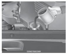
Do not overfill. Use a funnel to help prevent oil from being spilled on engine components. Use only the specified engine oil. (Refer to "Recommended lubricants and capacities" on page 8–9.)
