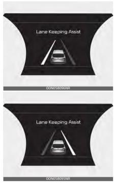
If the vehicle leaves a lane, the lane marker you cross will blink on the LCD display and the warning sound is provided.
