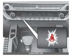
If you start to drive without the seat belt fastened or you unfasten the seat belt when you drive over 5 mph (9 km/h) and less than 12 mph (20 km/h), the corresponding warning light will illuminate. The warning light will turn off when the vehicle speed drops below 5 mph (9 km/h).
