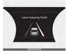
If the vehicle moves out its lane because steering torque for assistance is not enough, the line indicator of deviation direction will blink and the warning sound is provided.
