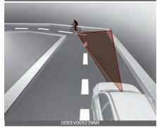
The performance of Forward Collision-Avoidance Assist may be limited when driving on a curved road.
