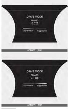
SMART mode selects the proper driving mode among ECO, COMFORT and SPORT by judging the driver's driving habits (i.e., mild or dynamic) from the brake pedal or the steering wheel operation.
