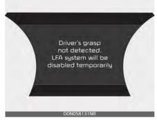
If the driver keeps hands off the wheel even with the hands-off warning on, the steering assist is temporarily deactivated automatically.
