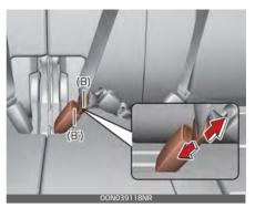
To retract the rear center seatbelt, insert the tongue plate into the web release hole (A'). Pull up on the seat belt web and allow the web- bing to retract automatically. Insert the tongue plate (A) into the hole on the belt assembly cover.
