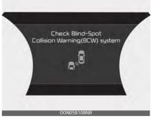
If there is a problem with Blind-Spot Collision Warning, a warning message will appear and the light on the switch will turn off. Blind-Spot Collision Warning will turn off automatically. Blind-Spot Collision-Avoidance Assist will not operate also if Blind-Spot Collision Warning turns off due to malfunction. In this case, have your vehicle inspected by an authorized Kia dealer.
