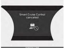
You must adjust the vehicle speed by depressing the accelerator or brake pedal according to the road condition and driving conditions. Always check the road conditions. Do not rely on the warning chime.
