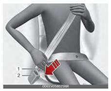
• Pull it out of the retractor and insert the metal tab (1) into the buckle (2).
