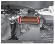
2. Unlock by turning the locking lever downward.
