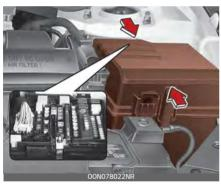
If the main fuse is blown, it must be removed as follows:
