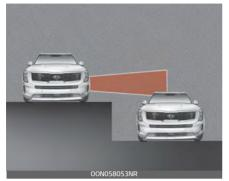
Blind-Spot Collision Warning and Blind-Spot Collision-Avoidance Assist may not operate properly when driving where the heights of the lanes are different.
