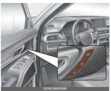
By saving the desired position into the system memory, different drivers can reposition the driver seat based upon their driving preference. If the battery is disconnected, the desired seat position memory will need to be re-saved.
