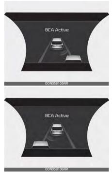
Blind-Spot Collision-Avoidance Assist may apply braking power, when an approaching vehicle is detected within a certain distance next to/behind your vehicle. Blind-Spot Collision-Avoidance Assist gently applies braking power on the tire that is located in the opposite side of the possibly-colliding point. The instrument cluster will inform the driver of Blind-Spot Collision-Avoidance Assist activation.
