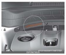
The number is punched on the engine compartment frame as shown in the drawing. To check the number, open the cover.
