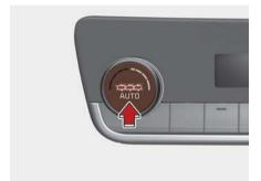
You can control the wind strength in three stages by pushing the AUTO button during automatic operation.
