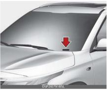
The VIN is also on a plate attached to the top of the dashboard. The number on the plate can easily be seen through the windshield from outside
