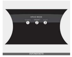
SMART mode: SMART mode automatically adjusts the driving mode (SMART ↔ SPORT) in accordance with the driver's driving habits.
