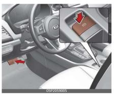
Releasing the parking brake with FPB switch.
