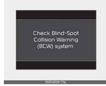
If there is a problem with BCW system, a warning message will appear. The system will turn off automatically. RCCW and RCCA will not operate also if BCW system turns off due to malfunction. You should have the vehicle inspected by an authorized Kia dealer.
