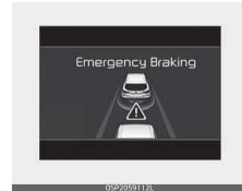
This warning message appears on the LCD display with a warning chime. Additionally, some vehicle system intervention occurs by the engine management system to help decelerate the vehicle. The brake control is maximized just before a collision, reducing impact when it strikes a forward vehicle.
