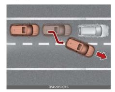
When driving in stop-and-go traffic, and a stopped vehicle in front of you merges out of the lane, FCA system may not immediately detect the new vehicle that is now in front of
