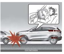
Front air bags are designed to inflate in a frontal collision depending on several factors, including the severity of impact of the front collision.
