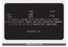
This label shows the maximum allowable weight of the fully loaded vehicle. This is called the GVWR (Gross Vehicle Weight Rating). The GVWR includes the weight of the vehicle, all occupants and cargo.
