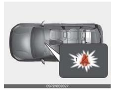
If you start to drive without the seat belt fastened over 5 mph (9 km/h) and less than 12 mph (20 km/h), the corresponding warning light will illuminate. The warning light will turn off when the vehicle speed drops below 5 mph (9 km/h).
