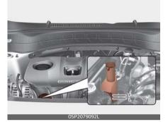
8. If the coolant level is low, add enough specified coolant to provide protection against freezing and corrosion. Bring the level to F,
