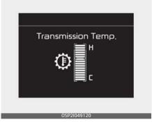
Try to drive so that the temperature gauge do not show high/ overheat. When the transmission is overheated, the warning message will display on the LCD. Follow the displayed message.
