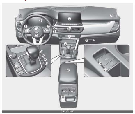
\* The actual shape may differ from the illustration. 1. Audio remote control button 4-156 2. Driver's front air bag 3-56 3. Horn 4-49 4. Cruise control / Smart Cruise Control system\* / LCD display control 5-102, 5-105, 4-58 button 5. Instrument cluster 4-53 6. Light control/Turn signals lever 4-99 7. Wiper and washer control lever 4-106 8. ENGINE START/STOP button 5-12 9. Audio, Video and Navigation\* 4-156 10.Hazard warning flasher 6-3 11.Climate control system 4-118, 4-124
