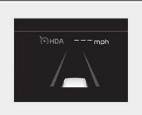
If both lanes are recognized properly (lane color: white), the steering wheel indicator ( ) lights up in green and then the steering control is initiated. When the system cannot provide temporary steering inputs, the indicator flashes green and then
