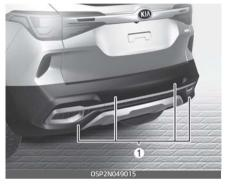
This system is a supplemental system that senses objects within the range and location of the sensors (1), it cannot detect objects in other areas where sensors are not installed.
