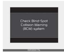
If there is a problem with BCW system, a warning message will appear. The system will turn off automatically. BCA will not operate also if BCW system turns off due to malfunction. You should have the vehicle inspected by an authorized Kia dealer.
