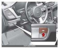
With the ignition switch in the ON position, LKA turns on automatically. The indicator ( in the cluster display will initially illuminate white. This indicates LKA system is in the READY but NOT ENABLED state.
