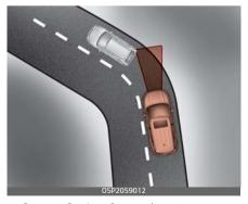
Smart Cruise Control system may not detect a moving vehicle in your lane, and then your vehicle could accelerate to the set speed. Also, the vehicle speed will decrease when the vehicle ahead is recognized suddenly.
