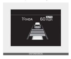
In the automatic speed setting mode, the set speed is automatically adjusted to the changing speed limits of highway sections.
