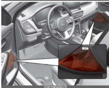
When the headlamp light is on, the ambient light is on at the same time Sound mood lamps (if equipped) could be set in the audio or infotainment menu.
