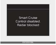
When the sensor lens cover is coverd with dirt, snow, or debris, SCC operation may stop temporarily. If this occurs, a warning message will appear on the LCD display. Remove any dirt, snow, or debris and clean the radar sensor lens cover before operating SCC.
