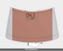
If there is heavy accumulation of snow on the front window, brush it off before operating the front glass heater. To activate the front glass heater:
