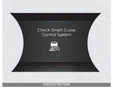
The message will appear when the vehicle distance control function is not functioning normally.
