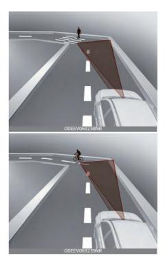
The performance of Forward Collision–Avoidance Assist may be limited when driving on a curved road.
