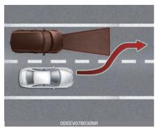
When a vehicle changes lanes in front of you, the smart regeneration system may not immediately detect the vehicle, especially if the vehicle changes lanes abruptly. In this case, you must maintain a safe braking distance, and if necessary, depress the brake pedal to reduce your driving speed in order to maintain a safe distance.
