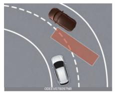
BCW may not operate properly when driving on a curved road. In certain instances, the function may not detect the vehicle in the next lane.
