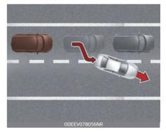
When driving in stop-and-go traffic, and a stopped vehicle in front of you merges out of the lane, FCA may not immediately detect the new vehicle that is now in front of you. In this case, you must maintain a safe
