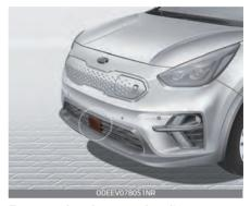
Front radar detects the distance to the vehicle ahead.
