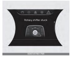
The message appears on the LCD display when the shifter dial is continuously stuck or there is problem with the shifter dial.
