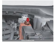
Replace any swollen or deteriorated hoses. The coolant level should be filled between F (MAX) and L (MIN) marks on the side of the coolant reservoir when motor compartment is cool. When the coolant level (in the reservoir) is low, have your vehicle inspected by an authorized Kia dealer. Use only designated coolant water for electric vehicles, adding other types of water or antifreeze can damage the vehicle.
