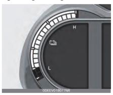
The SOC gauge shows the charging status of the high voltage battery. "L (Low)" position on the indicator indicates that there is not enough energy in the high voltage battery. "H (High)" position indicates that the driving battery is fully charged. When driving on highways or motorways, make sure to check in
