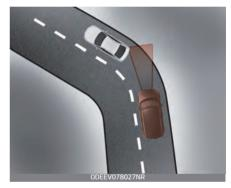
When driving on the curve, the system may not detect the vehicle in your lane and the regenerative braking level will reduce automatically, making you feel that the vehicle is accelerating.
