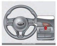
When Smart Cruise Control is not needed, press the Driving Assist button and deactivate the function.
