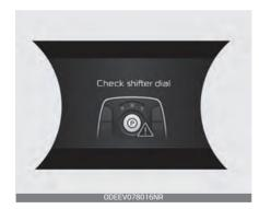
The message appears on the LCD display when there is problem with the shift buttons.
