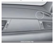
The indication of the system's presence are the letters "AIR BAG" located on the air bag pad cover on
