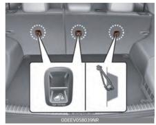
First secure the child restraint with the LATCH lower anchors or the seat belt. If the child restraint manufacturer recommends that the top tether strap be attached, attach and tighten the top tether strap to the top tether strap anchor.
