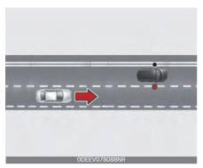
BCW feature will warn you when it detects a vehicle is approaching in an adjacent lane at a high rate of speed. If the driver activates the turn signal when the function detects an oncoming vehicle, the function sounds an audible warning.
