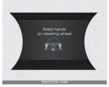
The hands-off warning appears when the function detects that the driver's hands are not on the steering wheel while HDA is in work.
