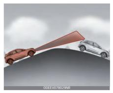
When driving uphill or downhill, the system may not detect the vehicle in your lane and the regenerative braking level will reduce automatically, making you feel that the vehicle is accelerating.
