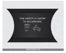
While Smart Cruise Control is in operation, your vehicle stops behind the vehicle in front when it stops. The message is displayed on the
