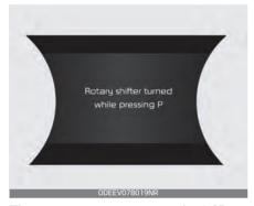
The message appears on the LCD display when the shift dial is not turned while pressing P button.
