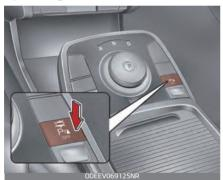
Press the Parking Distance Warning Off button to turn off the Reverse Parking Distance Warning. The indicator light on the button will turn on.
