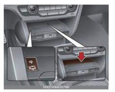
Firmly close all doors, and turn vehicle on. To start wireless charging, place the smart phone equipped with wireless charging function on the wireless charging pad.
