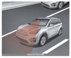
When the function detects the vehicle straying from its lane, it warn the driver with a visual and audible warning, while applying a slight counter steering torque, trying to prevent the vehicle from moving out of its lane.
