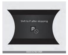
The message appears on the LCD display when the gear is shifted to P (Park) while the vehicle is moving.
