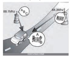
Multi-Path Cancellation - Radio signals being received from several directions can cause distortion or fluttering. This can be caused by a direct and reflected signal from the same station, or by signals from two stations with close frequencies. If this occurs, select another station until the condition has passed.
