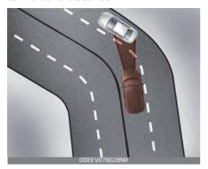
The smart regeneration system may recognize a vehicle in an adjacent lane when driving on a curved road. In this case, the system increase the braking level and slow the vehicle.
