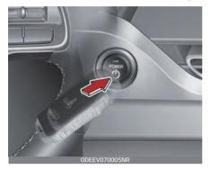
The side with the lock button should contact the POWER button directly.
