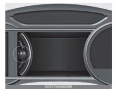
The additional distance to empty which is converted from the energy regenerated by the regenerative braking is displayed if the ECO/ECO+ mode is selected by pressing the Drive Mode button. The display is initialized to 0 if the regenerative braking stops because of acceleration. etc.
