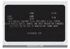
This label shows the maximum allowable weight of the fully loaded vehicle. This is called the GVWR (Gross Vehicle Weight Rating). The GVWR includes the weight of the vehicle, all occupants and cargo.
