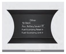
The driver can activate the Aux. Battery Saver+ function by placing the POWER button to the ON position and by selecting:
