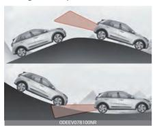
BCW may not operate properly when driving on a slope. In certain instances the function may not detect the vehicle in the next lane.
