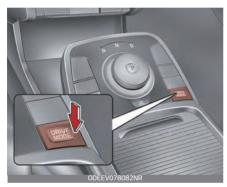
The mode changes, as below, whenever the DRIVE MODE button is pressed.
