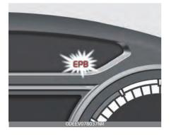
If the EPB malfunction indicator remains on, comes on while driving, or does not come on when the POWER button is changed to the ON position, this indicates that the EPB may have malfunctioned.
