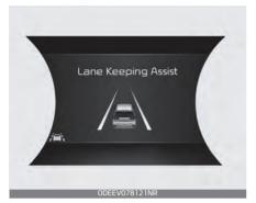
To see LKA screen on the LCD displau in the cluster. Tab to the Driving Assist mode ( ).
