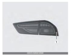
If the rear side marker (LED type) (1) does not operate, have the vehicle checked by an authorized Kia dealer.
