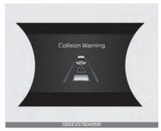
The warning message appears on the LCD display with the warning alarms.  FCA limitedly controls the brakes within certain limit to reduce the impact from the collision.
