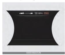
If temporary deceleration is required in the standby state and Navigation-based Smart Cruise Control is operating, the green (AUTO) symbol will illuminate on the cluster.
