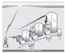
AM and FM radio signals are broadcast from transmitter towers located around your city. They are intercepted by the radio antenna on your vehicle. This signal is then processed by the radio and sent to your vehicle speakers. However, in some cases the signal coming to your vehicle may not be strong and clear.
