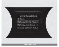
With the POWER button in the ON position, select or deselect "User settings → Driver Assistance→ Highway Driving Assist" on the LCD display to set whether or not to use each function.
