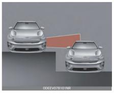
BCW may not operate properly when driving where the heights of the lanes are different.
