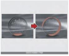
Immediately drive approximately 4~6 miles (7~10 km or, about 10 min) to evenly distribute the sealant in the tire. Do not exceed a speed of 50 mph (80 km/h). If possible, do not fall below a speed of 12 mph (20 km/h).
