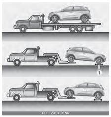
If you must tow the vehicle using only two wheels, lift the front wheels off the ground and tow the vehicle.
