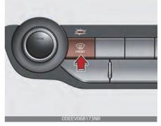
Most of the air flow is directed to the windshield with a small amount of air directed to the side window defrosters.
