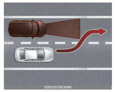
When a vehicle changes lanes in front of you, FCA may not immediately detect the vehicle, especially if the vehicle changes lanes abruptly. In this case, you must maintain a safe braking distance, and if necessary, depress the brake pedal to reduce your driving speed in order to maintain a safe distance.
