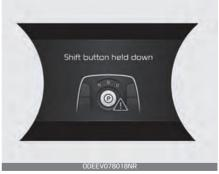
The message appears on the LCD display when the shifter button is continuously pressed or there is problem with the button.
