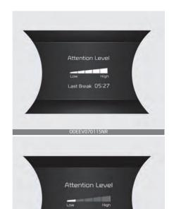
The driver's attention level is displayed on the scale of 1 to 5. The lower the level is, the more inattentive the driver is.
