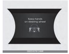
If the driver keeps hands off the wheel even with the hands-off warning on, the steering assist is temporarily released automatically.
