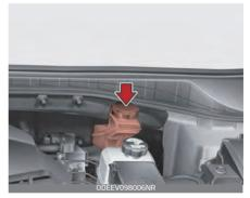
Before removing the reservoir cap and adding brake fluid, clean the area around the reservoir cap thoroughly to prevent brake fluid contamination.
