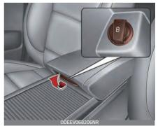
The electrical devices can be recharged when the power button is in ACC/ON position.
