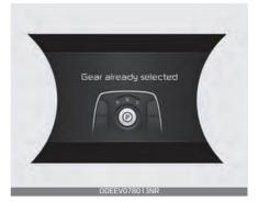
The message appears on the LCD display when the selected gear button is pressed again.
