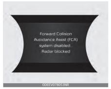
In this case, a warning message ("Forward Collision Avoidance Assist (FCA) system disabled. Radar blocked") will appear to notify the driver. Remove the foreign substances to allow FCA to function normally.
