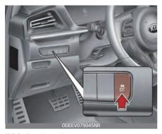
ESC checks where you are steering and where the vehicle is actually going. ESC applies the brakes on individual wheels and intervenes with the vehicle management system to stabilize the vehicle.
