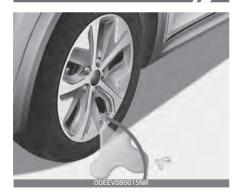
If the sealant is injected when the tire air pressure injection valve and sealant injection hose are not fully interlocked, the sealant may overflow and clog the valve.
