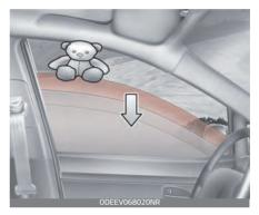
If the window detects the resistance while the power window switch is pulled up continuously, the window will stop upward movement then lower approximately 1 in (2.5 cm).
