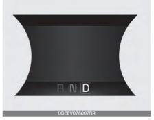
The indicator in the instrument cluster displays the gear position when the POWER button is in the ON position.
