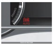
However, current regenerative braking level is maintained if the driver depresses the brake pedal while the system is in activation. Also, the system is cancelled temporarily if the accelerator pedal is depressed.
