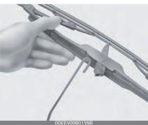
4. Install the blade assembly in the reverse order of removal.
