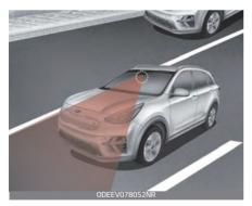
Front view camera is a sensor for detecting lanes and the front vehicles.
