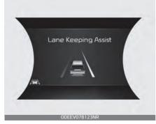
If the vehicle moves out its lane because steering torque for assistance is not enough, the lane indicator will blink.
