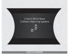
If there is a problem with BCW, a warning message will appear and the light on the button will turn off. The function will turn off automatically. RCCW will not operate also if BCW turns off due to malfunction. Have your vehicle inspected by an authorized Kia dealer.
