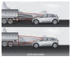
When the vehicle in front has heavy loading extended rearward, or when the vehicle in front has higher ground clearance, it may induce a hazardous situation. Always pay attention to road and driving conditions, while driving and, if necessary, depress the brake pedal to reduce your driving speed in order to maintain distance.
