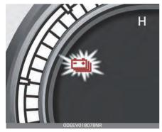
When the warning lamp turns ON the vehicle can drive an additional 12~18 miles (20~30 km) depending on the driving speed, heater/air conditioner, weather, driving style, an other factors. Charging is required.
