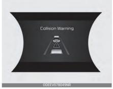
If there is a high risk of collision due to sudden braking of the front vehicle or lack of safety distance with the vehicle ahead during SCC driving, so that if the driver's brake or steering wheel operation is required, the Distance Step with the vehicle ahead will blink on the cluster and a collision warning will sound.
