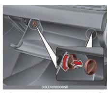
3. Remove the climate control air filter case by pulling out both sides of the cover.
