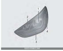
If the Low/High beam lamp (1), Low beam lamp (2), Front turn signal lamp (3), or side marker (4) does not operate, have the vehicle checked by an authorized Kia dealer.
