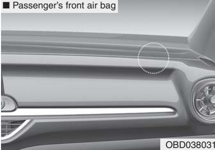
■ Passenger's front air bag
