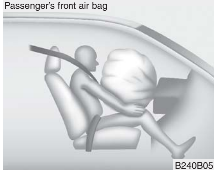
Passenger's front air bag
