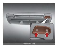
To change the rear fan speed, press the button () for higher speed, or press the button () for lower speed.
