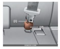
Pull out the tongue plate (B) from the pocket. Pull the tongue plate (B) and insert it into the buckle (B') until an audible "click" is heard, indicating the latch is locked.
