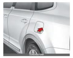
If the fuel filler lid does not open because ice has formed around it, tap lightly or push on the lid to break the ice and release the lid. Do not pry on the lid. If necessary, spray around the lid with an approved de-icer fluid (do not use radiator anti-freeze) or move the vehicle to a warm place and allow the ice to melt.
