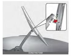
3. Make sure the blade assembly is installed firmly by trying to pull it slightly.
