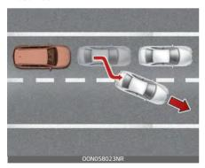
When driving in stop-and-go traffic, and a stopped vehicle in front of you merges out of the lane, the FCA may not immediately detect the new vehicle that is now in front of
