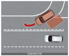
The BCW and BCA may not operate properly when driving where the road is merging/dividing. In certain instances the BCW/BCA may not detect the vehicle in the next lane. Always pay attention to road and driving conditions, while driving.
