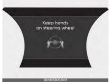
The hands-off warning appears when the system detects that the driver's hands are not on the steering wheel while the HDA is in work. (First warning: warning message, Second warning: warning message with warning sound)
