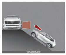
The RCCW/RCCA may not operate properly when the vehicle is on/near a slope.
