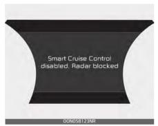
When the sensor lens cover is coverd with dirt, snow, or debris, the SCC operation may stop temporarily. If this occurs, a warning message will appear on the LCD display. Remove any dirt, snow, or debris and clean the radar sensor lens cover before operating the SCC.
