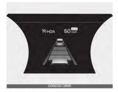
If the HDA operating conditions are all met and setting speed matches with the legal highway speed limit, the HDA will enter the automatic speed setting mode. (The set speed and the "AUTO" symbol will be displayed in green with an indicative sound)
