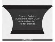
In this case, a warning message ("Forward Collision–Avoidance Assist (FCA) system disabled. Radar blocked") will appear to notify the driver.
