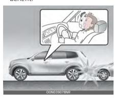
Front airbags may not inflate in side impact collisions, because passengers move in the direction of the collision. Thus, in side impacts, frontal airbag deployment would not provide additional occupant protection.
