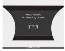
If you keep your hands off the wheel while driving with the LFA is in steering assist mode, the hands-off warning will be triggered.
