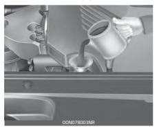
Do not overfill. Use a funnel to help prevent oil from being spilled on engine components. Use only the specified engine oil. (Refer to "Recommended lubricants and capacities" on page 8-6.)
