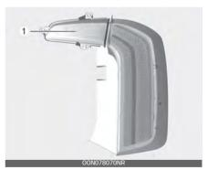
If the Back lamp bulb (Bulb Type) (1) does not operate, have your vehicle checked by an authorized Kia dealer.
