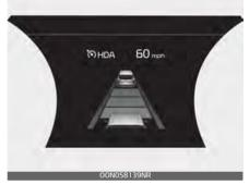
If the driver directly changes the speed, it enters the manual speed setting mode and the set speed is displayed in white and the "AUTO" symbol will disappear.
