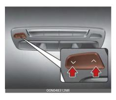
To change the rear air temperature, press the button (\sum ) for warmer air or press the button (\sum ) for cooler air.
