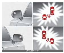
If a vehicle is detected within the boundary of the BCW, a warning light will illuminate on the outside rearview mirror and the Head-Up Display (if equipped).
