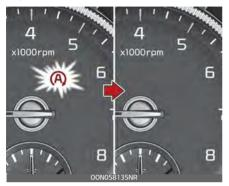
The engine will start and the green AUTO STOP indicator  $(\widehat{\mathbf{A}})$  on the instrument cluster will go out.
