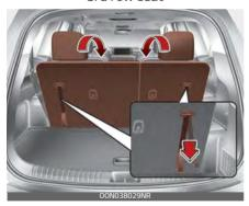
5. To use the rear seat, lift and pull the seatback backward by pulling on the folding lever (for 2nd row) or strap (for 3rd row). Pull the seatback firmly until it clicks into place. Make sure the seatback is locked in place.
