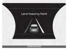
If the vehicle leaves a lane, the lane marker you cross will blink on the LCD display and the warning sound is provided.
