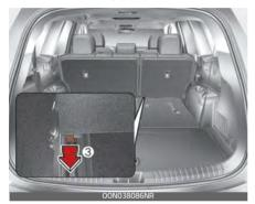
If the folding switch (1 or 2) in the 2nd row (in the upper part of the 2nd row seatback or the outer part of the seat) does not work, pull the strap (3) on the bottom left of the seat in the 2nd row. It works just like the folding switch and you can move the seat forward along with the seatback.
