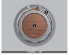
(A): Air discharged from [A] spreads over a wider area
