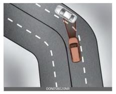
The FCA may recognize a vehicle in the next lane when driving on a curved road.
