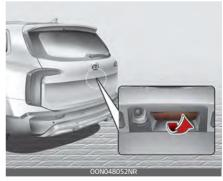
Only the liftgate is unlocked if the liftgate unlock button on the transmitter or smart key is pressed for approximately 1 second.
