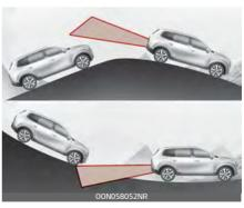
The BCW and BCA may not operate properly when driving on a slope. In certain instances the BCW/BCA may not detect the vehicle in the next lane.
