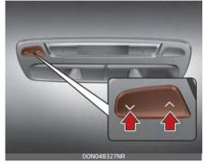
2. To change the temperature, press the button (\sums) for warmer air or press the button (\sums) for cooler air.
