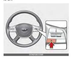
Select the appropriate distance according to road conditions and vehicle speed.
