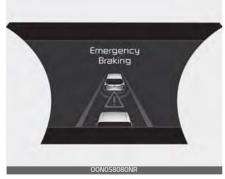
The warning message appears on the LCD display with the a warning chime.
