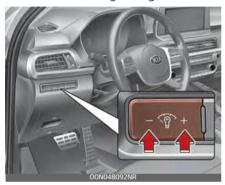
If the brightness reaches to the maximum or minimum level, an alarm will sound.
