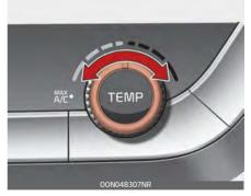
To change the air temperature in the passenger compartment, turn the knob to the right for warm and hot air or to the left for cooler air.
