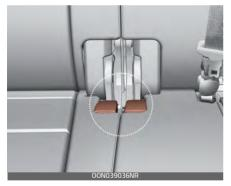
1. Route the seat belt webbing through the rear seat belt guides. It will help keep the belts from being trapped behind or under the seats.
