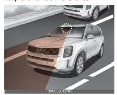
When the LKA system detects the vehicle straying from its lane, it alerts the driver with a visual and audible warning, while applying a slight countersteering torque, trying to prevent the vehicle from moving out of its lane.
