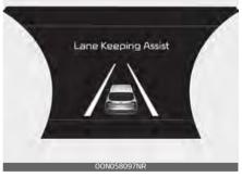
If the speed of the vehicle is over 40 mph (64 km/h) and the LKA detects lane markers, the color changes from gray to white.
