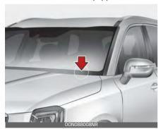
The VIN is also on a plate attached to the top of the dashboard. The number on the plate can easily be seen through the windshield from outside.
