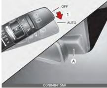
The rain sensor (A) located on the upper end of the windshield glass senses the amount of rainfall and controls the wiping cycle for the proper interval. The more it rains, the faster the wiper operates. When the rain stops, the wiper stops. To vary the speed setting, turn the speed control knob (1).
