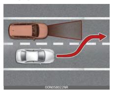
When a vehicle changes lanes in front of you, the FCA may not immediately detect the vehicle, especially if the vehicle changes lanes abruptly. In this case, you must maintain a safe braking distance, and if necessary, depress the brake pedal to reduce your driving speed in order to maintain a safe distance.
