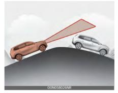
The FCA performance may be limited while driving upward or downward on a slope, and may not recognize the vehicle in front in the same lane. It may produce the warning message and the warning alarm prematurely, or it may not produce the warning message and the warning alarm at all.
