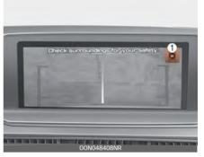
When you touch the icon (1), the top view is displayed on the screen and shows the distance from the vehicle in the back of your vehicle. Touch the icon (1) again, to switch back to the previous screen.
