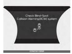
If there is a problem with the BCW, a warning message will appear and the light on the switch will turn off. The RCCW/RCCA will turn off automatically. RCCW and RCCA will not operate also if the BCW turns off due to malfunction. Have your vehicle inspected by an authorized Kia dealer.
