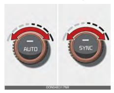
The temperature will increase to the maximum (HI) by turning the knob all the way to the right.
