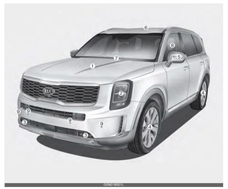
\* The actual shape may differ from the illustration. 1. Hood 4-40 2. Head lamp (Features of your vehicle) 4-109 Head lamp (Maintenance) 7-62 3. Front fog lamp (Features of your vehicle) 4-113 7-64 Front fog lamp (Maintenance) 4. Wheel and tire (Maintenance) 7-32 Wheel and tire (Specification) 8-5 4-61 5. Outside rearview mirror 6. Dual Sunroof 4-46
