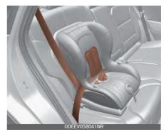
All passenger seat belts move freely under normal conditions and only lock under extreme or emergency conditions (emergency locking mode). So, in order to secure a child restraint, you must manually pull the seat belt all the way out to shift the retractor to the "automatic locking" mode.
