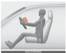
The front air bag modules are located both in the center of the steering wheel and in the front passenger's panel above the glove box. When the SRSCM detects a sufficiently severe impact to the front of
