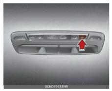
To turn off the rear climate control system, press the rear blower OFF button
