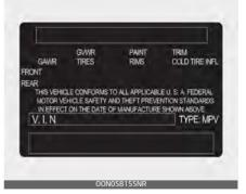
This label shows the maximum allowable weight of the fully loaded vehicle. This is called the GVWR (Gross Vehicle Weight Rating). The GVWR includes the weight of the vehicle, all occupants and cargo.
