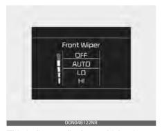
This indicator displays which wiper speed is selected using the wiper control.
