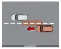
When the system detects an approaching vehicle, the rear doors will not unlock even if the driver attempts to unlock them using the electronic child safety lock button. The "Check surroundings then try again" warning message appears on the cluster and a warning sounds.
