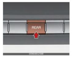
To turn off the rear climate control system, press the REAR button located on the front climate control panel and OFF button on the audio or multimedia screen.
