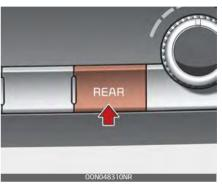
To turn off the rear climate control system, press the REAR button located on the front climate control panel and OFF button on the audio or multimedia screen.
