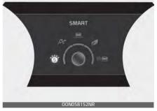
SMART mode: SMART mode automatically adjusts the driving mode (ECO ↔ COMFORT ↔ SPORT) in accordance with the driver's driving habits.
