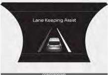
If the vehicle moves out its lane because steering torque for assistance is not enough, the line indicator of deviation direction will blink and the warning sound is provided.
