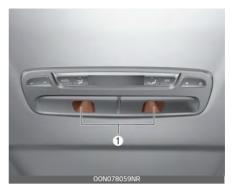
The LED lamps cannot be replaced as a single component because they are part of an integrated unit. The LED lamps have to be replaced with the unit.
