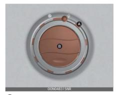
(A): Air discharged from [A] spreads over a wider area.
