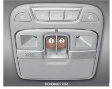
The sunroof can only be opened, closed, or tilted when the ENGINE START/STOP button is in the ON position.
