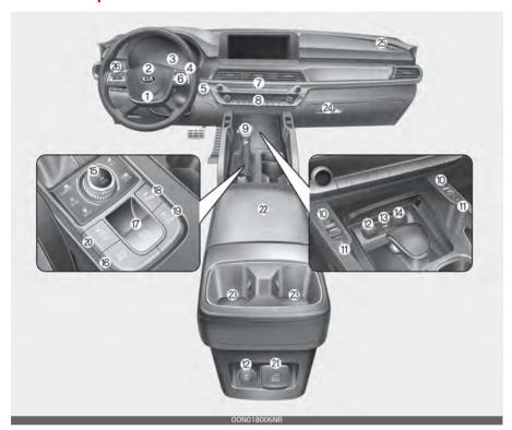
\* The actual shape may differ from the illustration. 1. Driver's front air bag 3-65 4-54 2. Horn 3. Instrument cluster 4-64 4. Wiper and washer control lever 4-116 5. ENGINE START/STOP button 5-9 6. Smart Cruise Control with Stop & Go 5-72 7. Hazard warning flasher 6-3 8. Climate control system 4-129, 4-138 9. Shift lever 5-13 10. Front seat warmer switch 4-157 11.Front seat air ventilation switch 4-158 12.Power outlet 4-160 13.USB port 4-172
