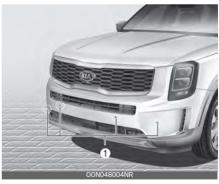
The sensing range and objects detectable by the sensors (1) are limited. Whenever moving while using the parking distance warning, pay as much attention to what is in
