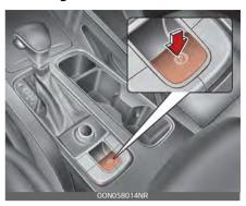
Releasing the parking brake with EPB switch,
