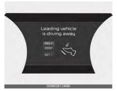
If the driver does not take action for a certain period of time after the vehicle in front departs, the message is displayed on the cluster. The vehicle departs automatically if the accelerator pedal is depressed or [RES +] or [SET -] switch is activated when there is a vehicle in front.
