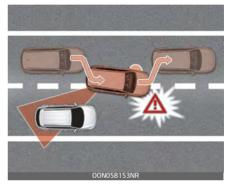
The BCA may activate the Electronic Stability Control (ESC) in accordance with a colliding possibility with an approaching vehicle while changing lanes.
