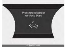
If you move the transmission lever from N to D (Manual mode) or R without depressing the brake pedal after stopping engine automatically, the engine does not restart automatically and a warning chime alarms. When this happens, press the brake pedal for auto start.
