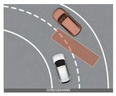
The BCW and BCA may not operate properly when driving on a curved road. In certain instances the system may not detect the vehicle in the next lane.
