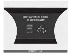
While the SCC is in operation, your vehicle stops behind the vehicle in front when it stops. The message is displayed on the cluster within 3 seconds after the stop and the system will be in the standby position.
