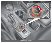
You can switch from DRIVE MODE to SNOW mode by turning the knob.
