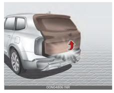
During power opening and closing if the power liftgate is blocked by an object or part of the body, the power liftgate will detect the resistance.  If the resistance is detected while opening the liftgate, it will stop and move in the opposite direction.
