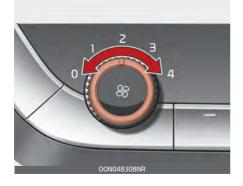
Setting the fan speed control knob to the "0" position turns off the fan.
