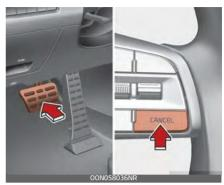
The SCC is temporarily canceled when the brake pedal is depressed or the CANCEL button is pressed.
