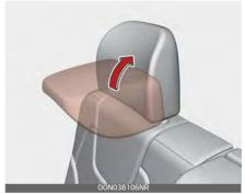
The headrest will fold down automatically when folding the seatback.
