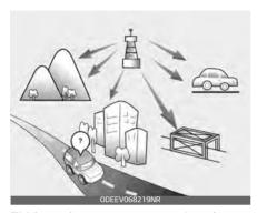
FM broadcasts are transmitted at high frequencies and do not bend to follow the earth's surface. Because of this, FM broadcasts generally begin to fade within short distances from the station. Also, FM signals are easily affected by buildings, mountains, and obstructions. This can lead to undesirable or unpleasant listening conditions which might lead you to believe a problem exists with your radio.
