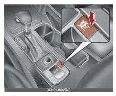
This system activates when the parking distance warning button is pressed with the ENGINE START/STOP button ON.
