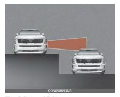
The BCW and BCA may not operate properly when driving where the heights of the lanes are different. In certain instances, the BCW/BCA may not detect the vehicle on a road with different lane heights (underpass joining section, grade separated intersections, etc.). Always pay attention to road and driving conditions, while driving.
