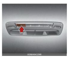
To turn off the rear climate control system, press the rear blower OFF button
