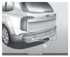
This system is a supplemental system and it is not intended to nor does it replace the need for extreme care and attention of the driver. The sensing range and objects detectable by the back sensors (1) are limited. Whenever backing-up, pay as much attention to what is behind you as you would in a vehicle without a parking distance warning-reverse.
