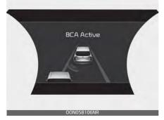
The BCA may apply braking power, when an approaching vehicle is detected within a certain distance next to/behind your vehicle.
