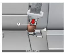
Do not separate the mini tongue (1) and mini buckle (2) even if there is not an occupant.
