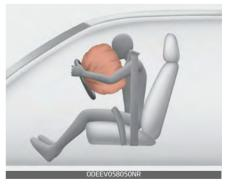
A fully inflated airbag (with a properly fastened seat belt) slows the forward motion of the driver or passenger, reducing the risk of head and chest injury.
