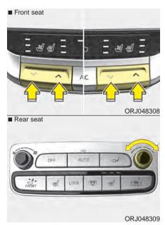
Press the temperature buttons or turn the temperature control knob to the desired temperature.
