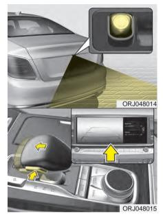
Rear View Monitor system will activate with the ignition switch ON, engine ON and the shift lever in the R (Reverse) position.
