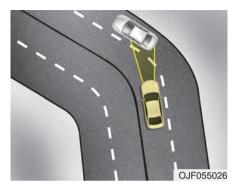
FCA system may recognize a vehicle in the next lane when driving on a curved road.
