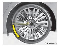
7. Loosen the wheel lug nuts counterclockwise one turn each, but do not remove any nut until the tire has been raised off the ground.
