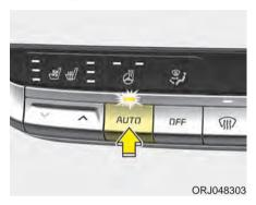
Press the AUTO button. The modes, fan speeds, air intake and air-conditioning will be controlled automatically by setting the temperature.
