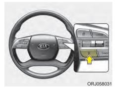
When SCC system is ON, you can set and maintain the distance to the vehicle ahead without pressing the accelerator or brake pedal.
