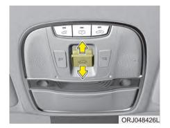
The sunshade will automatically open with the glass panel when the glass panel moves. Close it manually if you want it closed.
