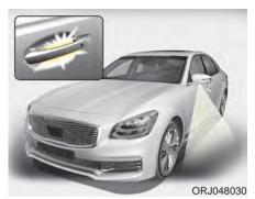
When all the doors (and trunk) are locked and closed, the pocket lamp and puddle lamp will come on for about 15 seconds if any of the below is performed.
