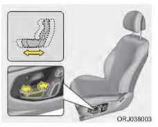
Push the control switch forward or backward to move the seat to the desired position.
