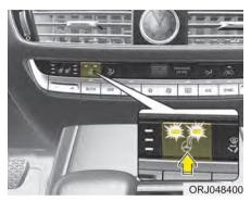
When the Engine Start/Stop Button is in the ON position, pressing the heated steering wheel button warms the steering wheel. The indicator on the button will illuminate.
