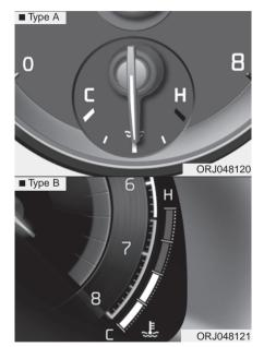
This gauge indicates the temperature of the engine coolant when the Engine Start/Stop button is ON.
