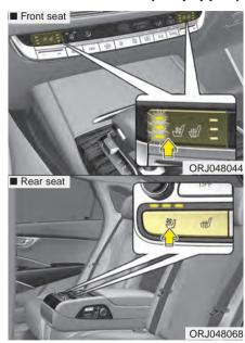
The temperature setting of the seat changes according to the switch position.
