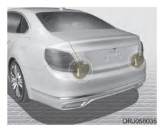
The rear radars are the sensors inside the rear bumper for detecting the side/rear areas. Always keep the rear bumper clean for proper operation of the system.
