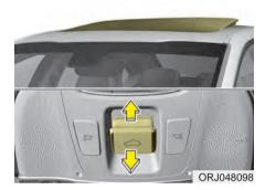
To tilt open the sunroof, push the sunroof control lever upward. To stop the sunroof tilting at any point, operate the control lever.
