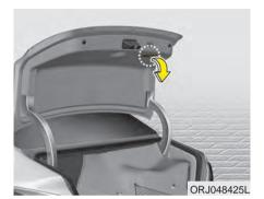
To close, lower the trunk lid, then press down on it until it locks. To be sure the trunk lid is securely fastened, always check by trying to pull it up again.
