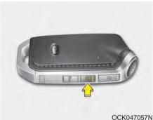
The power trunk will open automatically by doing one of the following:
