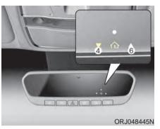
5.If the both indicator (4) and (6) are flashing rapidly for about 5 seconds, the two way synchronization is completed.
