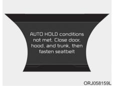
When you press the [AUTO HOLD] switch, if the driver's door and engine hood are not closed or the driver's seat belt is unfastened, a warning will sound and a message will appear on the LCD display. At this moment, press the [AUTO HOLD] button after closing the driver's door and engine hood and fastening the seat belt.
