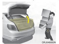
On a vehicle equipped with a smart key, the trunk lock is released with no-touch activation using the Smart Trunk system.
