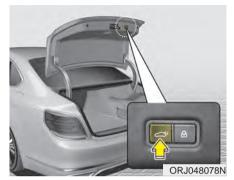
Press the power trunk close button for approximately one second when the trunk is opened.
