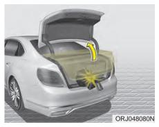
During power opening and closing if the power trunk is blocked by an object or part of the body, the power trunk will detect the resistance.
