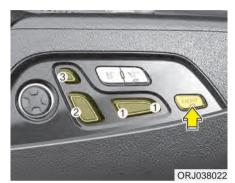
Press Front button (Switch ON) to adjust the seat position. You can adjust the forward/backward movement (1) of the front passenger seat, its angle (2), and the height of the headrest (3). If you press the button again to switch off, you can adjust the rear right passenger seat.
