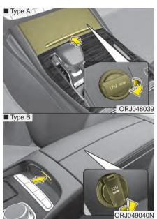
The power outlet is designed to provide power for mobile telephones or other devices designed to operate with vehicle electrical systems. The devices should draw less than 20 amps with the engine running.
