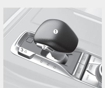
When you move the shift lever (1), depress the brake pedal while pressing the UNLOCK button (2).
