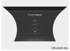
When the wiper switch is operated, the corresponding mode is displayed.
