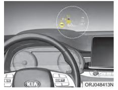
The head up display is a transparent display which projects a shadow of some information from the instrument cluster and navigation on the windshield glass.
