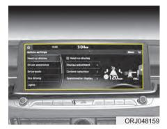
The HUD display will be activated or deactivated in Setup mode while engine is ON.
