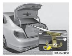
Pull the strap (1) to hang a bag on the hook (2). Fold the hook when not in use.
