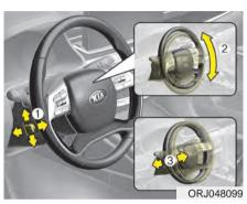
Adjust the steering wheel angle (2) and position (3) with the switch (1).
