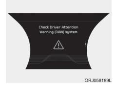
When the "Check System" warning message appears, the system is not working properly. If this occurs, have the system checked by an authorized K900 Kia dealer
