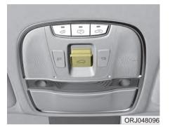
If your vehicle is equipped with a sunroof, you can slide or tilt your sunroof with the sunroof control lever located on the overhead console.
