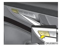
If you open the door with the DOOR switch on, the seat will be moved backwards. (However, this function does not work if the seat is already at its farthest rear position.) When the door is closed, the seat will move forward. The switch can be turned on and off.
