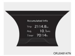
Displays accumulated information starting from a mileage/fuel efficiency/time default point.
