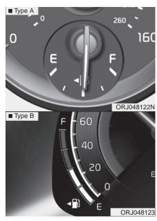
This gauge indicates the approximate amount of fuel remaining in the fuel tank.
