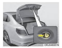
Your vehicle is equipped with an emergency trunk safety release lever located inside the trunk. In the event that someone is inadvertently locked in the trunk, the trunk can be opened by moving the lever in the direction of the arrow and pushing open the trunk.
