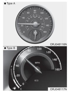
The speedometer indicates the speed of the vehicle and is calibrated in miles per hour (mph) and/or kilometers per hour (km/h).
