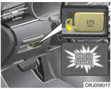
To apply the EPB (electronic parking brake):
