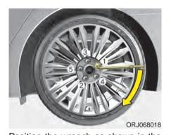
Position the wrench as shown in the drawing and tighten the wheel nuts. Be sure the socket is seated completely over the nut. Do not stand on the wrench handle or use an extension pipe over the wrench handle. Go around the wheel, tightening every nut following the numerical sequence shown in the image until they are all tight. Double-check each nut for tightness. After changing wheels, have an authorized K900 Kia dealer tighten the wheel nuts to their proper torque as soon as possible.
