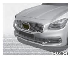
Smart Cruise Control (SCC) system uses a sensor to detect distance to the vehicle ahead.
