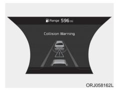
This warning message appears on the LCD display with a warning chime. Additionally, the engine management system intervenes to help decelerate the vehicle.
