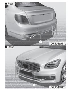
The Parking Distance Warning system assists the driver during movement of the vehicle by chiming if any object is sensed within the distance of 39 in. (100 cm) in front and 47 in. (120 cm) behind the vehicle.
