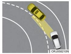
BCW and BCA systems may not operate properly when driving on a curved road. In certain instances, the system may recognize a vehicle in the same lane.
