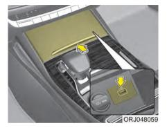
You can use an USB port to plug in an USB or iPod®.
