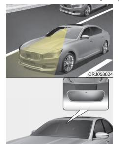
Lane Keeping Assist (LKA) system is designed to detect the lane markers on the road with a front view camera at the front windshield, and assists the driver's steering to help keep the vehicle in the lanes
