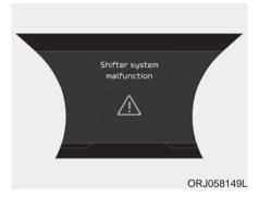
The warning message appears on the LCD display, when the transmission or the shift lever does not properly operate in the P (Park) position. If this occurs, have the vehicle inspected by an authorized K900 Kia dealer immediately.
