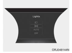
When you activate the headlamp switch, the corresponding mode is displayed.
