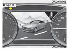
BVM (Blind-Spot View Monitor) system displays the rear and side views of the vehicle on a center cluster screen upon the driver's activation of the turn signal.
