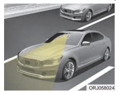
Lane Following Assist (LFA) system helps detect lane markers on the road with a front view camera at the front windshield, and assists the driver's steering to help keep the vehicle between lanes.
