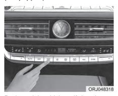
During night driving, if hands are near to touch the climate control system, button lighting will increase for better recognition. Switch lighting function can be selected or deselected on the audio display. Hands in gloves are not recognized for this function.
