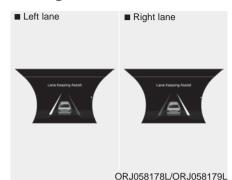
If the vehicle leaves a lane or road edge, the lane marker you cross will blink on the LCD display and the warning sound is provided.
