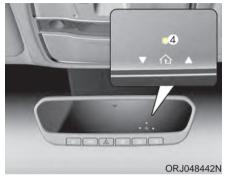
4. Press the Original Transmitter (OT) button until the indicator (4) is turned continuously ON or flashes in Green for approximately 10 seconds and it indicates the programming is completed.
