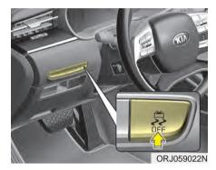
Electronic Stability Control (ESC) system is designed to stabilize the vehicle during cornering maneuvers. ESC checks where you are steering and where the vehicle is actually going. ESC applies the brakes on individual wheels and intervenes with the engine management system to stabilize the vehicle.
