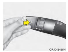
To turn on the high beam headlamp, push the lever away from you. The lever will return to its original position. The high beam indicator will illuminate when the headlight high beams are switched on.
