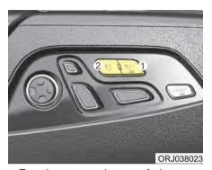
For the convenience of the passenger sitting in the rear right passenger's seat, the seat allows a person to adjust both the rear right passenger's seat and the front passenger seat by operating the rear right passenger's seat switches. But the rear relaxation seat system doesn't work if a person is sitting in the front passenger seat or the door of front passenger seat is opened.
