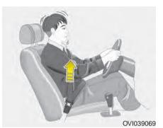
The purpose of the pre-active seat belt is to prevent passengers from getting hurt by tightening the seat belt right before a collision or dangerous maneuver.
