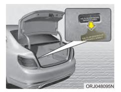
If the fuel filler lid does not open using the fuel filler lid opener button, you can open it manually.
