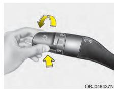
High Bean Assist (HBA) system is a system that automatically adjusts the headlamp range (switches between high beam and low beam) according to the brightness of other vehicles and road conditions.
