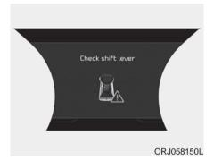
The warning message appears on the LCD display when there is a malfunction with one of the key transmission components.
