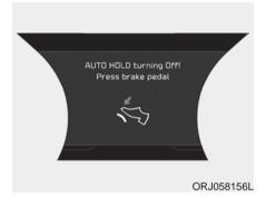
When the conversion from Auto Hold to EPB is not working properly, a warning will sound and a message will appear.
