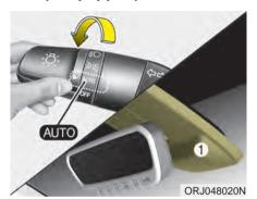
Low Beam Assist (LBA) system uses the steering angle and vehicle speed to keep your field of vision wide by swiveling and leveling the headlamp. Change the switch to the AUTO position when the engine is running. Low Beam Assist (LBA) system will operate when the headlamp is ON. To turn off LBA system change the switch to other positions. After turning LBA system off, headlamp swiveling no longer occurs, but leveling operates continuously.
