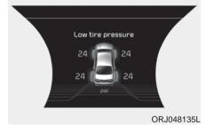
When the tire pressure monitoring system warning indicators are illuminated, one or more of your tires is significantly under-inflated.
