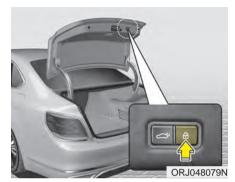
▶ Power trunk Lock button operation Press the Lock button on the trunk while carrying the Smart Key with all the vehicle's doors closed.
