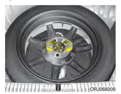
Turn the tire hold-down wing bolt counterclockwise.
