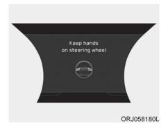
The hands-off warning appears when the system detects that the driver's hands are not on the steering wheel while HDA system is in work. (First warning: warning message, Second warning: warning message with warning sound)
