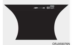
If both lanes are recognized properly (lane color: white), the steering wheel indicator ( ) lights up in green and then the steering control is initiated.
