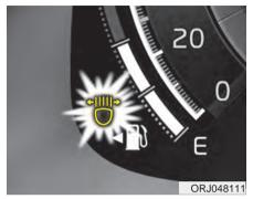
If LBA system malfunction indicator comes on, LBA system is not working properly. Drive to the nearest safe location and restart the engine. If the indicator continuously remains on, have your vehicle checked by an authorized K900 Kia dealer as soon as possible.
