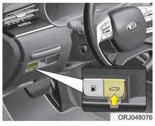
Press the power trunk close button for approximately one second when the trunk is opened.
