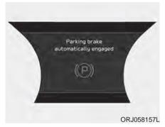
If the EPB is applied while Auto Hold is activated because of an ESC (Electronic Stability Control) signal, a warning will sound and a message will appear.
