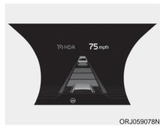
If the driver directly changes the speed, it enters the manual speed setting mode and the set speed is displayed in white and the "AUTO" symbol will disappear.
