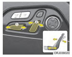
The control switch (1) works in conjunction with the control switch (2). Also, the seatback angle adjustment and the forward/backward adjustment are made at the same time.
