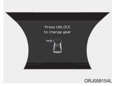
The warning message appears on the LCD display when the [UNLOCK] button is not pressed while shifting the gear.
