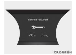
When Service Required is set, the remaining distance/time before service is required appears on the LCD screen.
