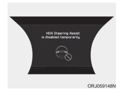
If you keep your hands off the steering wheel even with the hands-off warning on, the steering assist and Smart Cruise Control will be temporarily released automatically.
