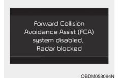
When the sensor is covered or the sensor lens is dirty with foreign substances, such as snow or rain, the FCA system may not be able to detect vehicles. In this situation, a warning message ("Forward Collision-Avoidance Assist (FCA) system disabled. Radar blocked") will appear to notify the driver. Remove the foreign substances to allow the FCA system to function property.
