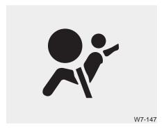
The purpose of the air bag warning light in your instrument panel is to alert you of a potential problem with your air bag system, which could include your side and/or curtain air bags used for rollover protection.
