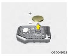
A battery should last for several years, but if the transmitter or smart key is not working properly, try replacing the battery with a new one. If you are unsure how to use or replace the battery, contact an authorized Kia dealer.
