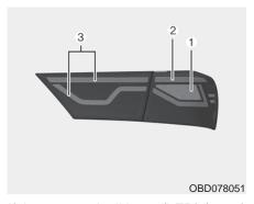
If the stop and tail lamp (LED) (1,2,3) does not operate, have the vehicle checked by an authorized Kia dealer.
