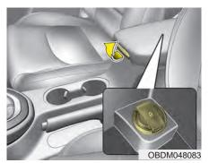
The USB car charger allows drivers to charge their digital devices their digital devices such as smartphones and tablets. Connect the device to the USB port using a manufacturer certified cable to begin charging.
