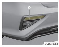
If the rear turn signal lamp (1) does not operate, have the vehicle checked by an authorized Kia dealer.
