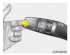
To flash the headlights, pull the lever towards you. It will return to the normal (low beam) position when released. The headlight switch does not need to be on to use this flashing feature.
