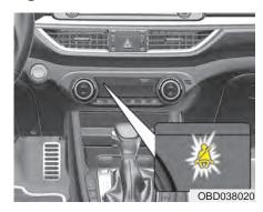
When the ignition switch is ON or the engine starts with the front passenger seat belt unfastened, the warning light will stay on until the belt is fastened. When the ignition switch is ON or the engine starts with the front passenger seat belt fastened, the warning light will stay for about 6 seconds.
