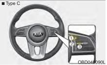
The LCD window modes can be changed by using the control buttons on the steering wheel.
