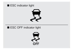
When the ignition switch is turned to ON, the indicator light illuminates, then goes off if the ESC system is operating normally.
