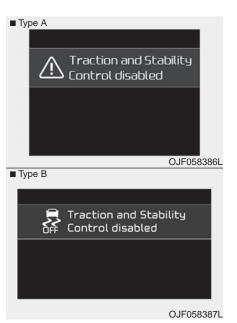
In this state, the car stability control function will not operate.
