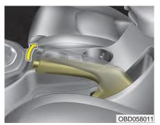
Check the stroke of the parking brake by counting the number of "clicks" heard while fully applying it from the released position. Also, the parking brake alone should securely hold the vehicle on a fairly steep grade. If the stroke is more or less than specified, have the parking brake adjusted by an authorized Kia dealer.
