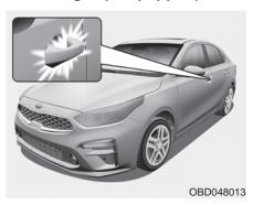
When all the doors (and tailgate) are locked and closed, the door handle lamp will come on for about 15 seconds if any of the below is performed.
