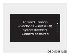
When the sensor is covered or the sensor lens is dirty with foreign substances, such as snow or rain, the FCA system may not be able to detect vehicles. In this situation, a warning message ("Forward Collision-Avoidance Assist (FCA) system disabled. Camera blocked") will appear to notify the driver. Remove the foreign substances to allow the FCA system to function property.
