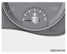
The fuel gauge indicates the approximate amount of fuel remaining in the fuel tank. The fuel tank capacity is indicated in Chapter 8. The fuel gauge is supplemented by a low fuel warning light, which will illuminate when the fuel tank is nearly empty.
