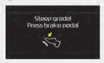
This warning message is displayed when the vehicle is driven slowly on a grade and the vehicle detects that the brake pedal is not applied.
