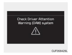
When the "Check System" warning message appears, the system is not working properly. In this situation, take your vehicle to an authorized Kia dealer and have the system checked.
