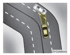
Your vehicle speed can be reduced due to a vehicle in the adiacent lane. Adjust your vehicle speed by depressing the brake pedal according to the road and driving conditions ahead. Apply the accelerator pedal and select the appropriate set speed. Check to be sure that the road conditions permit safe operation of the smart cruise control.
