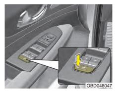
The driver can disable the power window switches on the rear passengers' doors by pressing the power window lock switch to the lock position (pressed).
