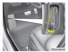
Pull the release lever to unlatch the hood. The hood should pop open slightly.
