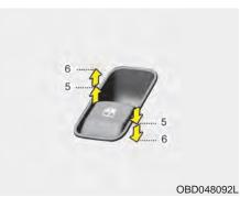
Pressing or pulling up the power window switch momentarily to the second detent position (6) completely lowers or lifts the window even when the switch is released. To stop the window at the desired position while the window is in operation, pull up or press and release the switch to the opposite direction of the movement. If the power window is not operated correctly, the automatic power window system must be reset as follows:
