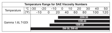
For Fuel economy, it is recommended to use the engine oil of a viscosity grade SAE 5W-30 (API Latest (ILSAC Latest) or ACEA A5/B5). However, if the engine oil is not available in your country, select the proper engine oil using the engine oil viscosity chart.
