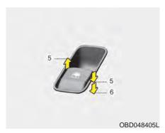
Pressing the power window switch momentarily to the second detent position (6) completely lowers the driver's window even when the switch is released. To stop the window at the desired position while the window is in operation, briefly pull up the switch to the opposite direction of the window movement.
