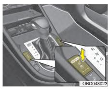
The seat warmer is provided to warm the front seats during cold weather. With the ignition switch in the ON position, push either of the switches to warm the driver's seat or the front passenger's seat. During mild weather or under conditions where the operation of the seat warmer is not needed, keep the switches in the "OFF" position.
