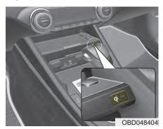
The wireless smart phone charging system is located in front of the center console.
