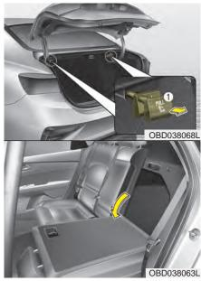
3. Pull out the seatback locking knob(1) in the trunk, then fold the seat toward the front of the vehicle.
