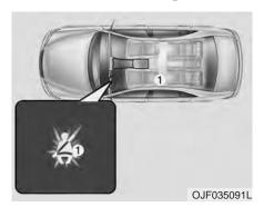
If a driver turns the ignition switch ON or the engine starts with the seat belt unfastened, the seat belt warning light will stay on until the driver fastens the seat belt and the warning sound will continue for 6 seconds. If a driver turns the ignition switch ON or the engine starts with seatbelt fastened, the warning light will stay for 6 seconds and the warning sound will not be heard
