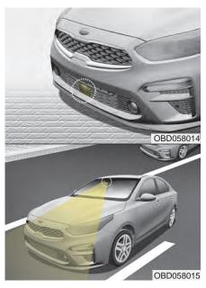
By detecting the vehicle or pedestrian ahead of the vehicle, the sensor helps to operate the Forward Collision-Avoidance Assist when the vehicle is at risk of a collision.
