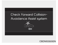
When the FCA is not working properly, the FCA warning light ( ) will illuminate and the warning message will appear for a few seconds. After the message disappears, the master warning light ( ) will illuminate. In this situation, have the vehicle inspected by an authorized Kia dealer.
