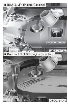
If it is near or at L, add enough oil to bring the level to F. **Do not overfill.**
