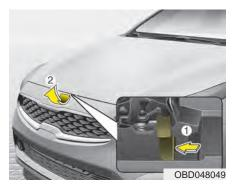
Go to the front of the vehicle, raise the hood slightly, push the secondary latch (1) inside of the hood center and lift the hood (2).
