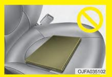
Do not place electronic devices such as laptops, DVD players, or conductive materials such as water bottles on the passenger seat.
