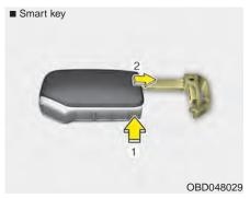
To remove the mechanical key, press and hold the release button and remove the mechanical key.
