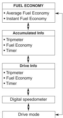
To change the trip mode, scroll the MOVE scroll switch  $(\land/\lor)$  or press the TRIP button in the trip computer mode.
