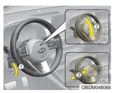
To change the steering wheel angle, pull down the lock release lever (1), adjust the steering wheel to the desired angle (2) and height (3), then pull up the lock-release lever to lock the steering wheel in place. Be sure to adjust the steering wheel to the desired position before driving.
