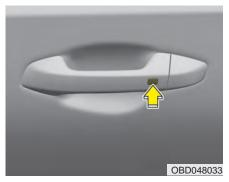
Pressing the button of the front outside door handles with all doors closed and any door unlocked, locks all the doors.
