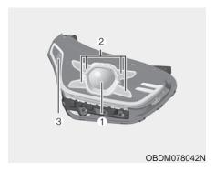
If the Low/High beam lamp(1), Day time running lamp/Position lamp(2), side marker(3) do not operate, have the vehicle checked by an authorized Kia dealer.
