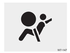
If the air bag warning light is illuminated for more than 6 seconds after the Engine Start/Stop button is turned on, or of it illuminates during vehicle operation, an SRS component may not be functioning properly and you should have your vehicle checked by an authorized Kia dealer.
