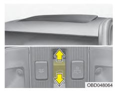
To tilt open the sunroof, push the sunroof control lever upward until the sunroof moves to the desired position.
