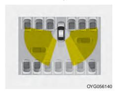
When your vehicle moves backwards from a parking position, the sensor detects approaching vehicles to the left or right side and gives information to the driver
