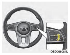
Move the lever down (to SET-), and release it at the desired speed. The SET speed on the LCD screen will appear. Release the accelerator at the same time. The desired speed will automatically be maintained.
