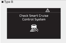
The message will appear when the vehicle to vehicle distance control system is not functioning normally.
