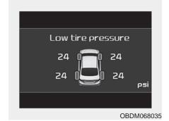
When the tire pressure monitoring system warning indicators are illuminated, one or more of your tires is significantly under-inflated.
