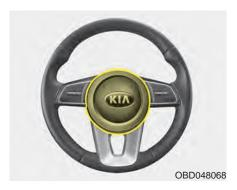
To sound the horn, press the horn symbol on your steering wheel. Check the horn regularly to be sure it operates properly (see illustration).
