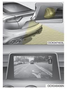
The rear view monitor will activate with the ignition switch ON, engine ON and the shift lever in the R (Reverse) position.
