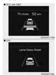
This mode displays the state of the Smart Cruise Control with Stop & Go and Lane Keeping Assist (LKA).
