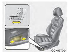
Push the control switch forward or backward to move the seat to the desired position. When the control switch is operated forward, the seat cushion is slightly raised, and the seat cushion lowered when the switch is operated backward.
