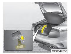
If the fuel filler lid does not open using the fuel filler lid opener button, vou can open it manually.
