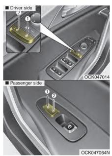
Operate by pressing the central door lock switch.
