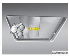
If an object or part of the body is detected while the sunroof is closing automatically, it will reverse the direction, and then stop.
