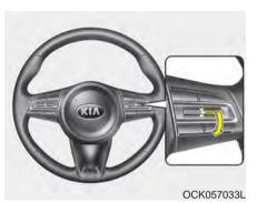
3. Move the lever down (to SET-), and release it at the desired speed. The cruise indicator and set speed on the LCD screen will illuminate. Release the accelerator at the same time. The desired speed will automatically be maintained.
