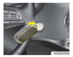
If the smart key battery is weak or the smart key does not work correctly, you can start the engine by pressing the engine start/stop button with the smart key.
