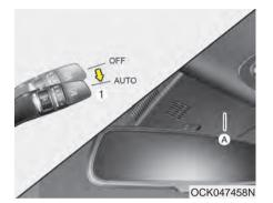
The rain sensor (A) located on the upper end of the windshield glass senses the amount of rainfall and controls the wiping cycle for the proper interval. The more it rains, the faster the wiper operates. When the rain stops, the wiper stops.
