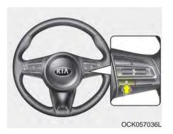
This function allows you to program the vehicle to maintain relative distance to the vehicle ahead without depressing the accelerator pedal or brake pedal. The vehicle to vehicle distance will automatically activate when the smart cruise control system is on.
