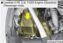
The air filter must be replaced when necessary, and should not be washed
