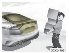
On a vehicle equipped with a smart key, the liftgate can be opened with no-touch activation using the Smart Liftgate system. How to use the Smart Liftgate
