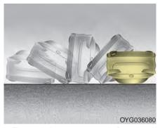
Front air bags may not inflate in all rollover accidents where the SRSCM indicates that the front air bag deployment would not provide additional occupant protection.
