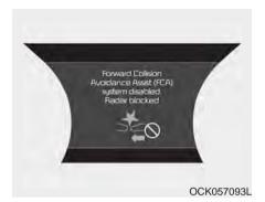
When the sensor is covered or the sensor lens is dirty with foreign substances, such as snow or rain, the FCA system may not be able to detect vehicles or pedestrians. In this case, a warning message ("Forward Collision Avoidance Assist (FCA) system disabled. Radar blocked") will appear to notify the driver. Remove the foreign substances to allow the FCA system to function.
