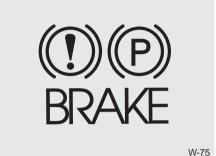
Check the brake warning light by turning the ignition switch ON (do not start the engine). This light will be illuminated when the parking brake is applied with the ignition switch in the START or ON position.
