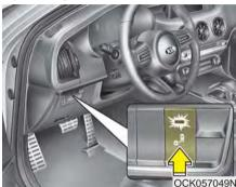
The indicator on the switch will illuminate when the Blind-Spot Collision Warning System (BCW) switch is pressed with the engine start/stop Rutton ON
