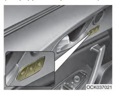
Driver Position Memory System is the facility that enables driver's seat, leg extension, steering wheel, exterior mirrors, cluster and head-up display (HUD) to be controlled with a simple button operation, which allows a driver to recall memorized driving positions and automatically control them.
