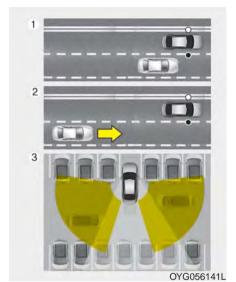
The Blind-Spot Collision Warning (BCW) system uses radar sensors in the rear bumper to monitor and warn the driver of an approaching vehicle in the driver's blind spot area.
