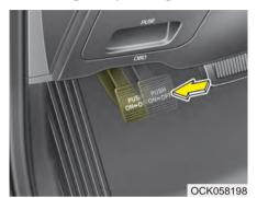
Check whether the stroke is within specification when the parking brake pedal is depressed with 44 lbs, 196 N (20 kg) of force. Also, the parking brake alone should securely hold the vehicle on a fairly steep grade. If the stroke is more or less than specified, have the parking brake adjusted by an authorized Kia dealer.
