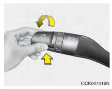
The High Beam Assist is a system that automatically adjusts the head-lamp range (switches between high beam and low beam) according to the brightness of other vehicles and road conditions.
