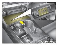
You can use an AUX port to connect audio devices and a USB port to plug in a USB or iPod®.
