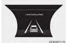
If the speed of the vehicle is over 40 mph (64 km/h) and the system detects lane markers, the color changes from gray to white. When the conditions below are met, LKA system will be enabled to assist steering.
