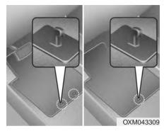
When using a floor mat on the front floor carpet, make sure it attaches to the floor mat anchor(s) in your vehicle. This keeps the floor mat from sliding forward.
