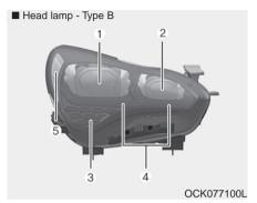
If the Low/High beam lamp (1, 2), Front turn signal lamp (3), Day time running lamp/Position lamp (4), and/or Side marker (5) do not operate, have the vehicle checked by an authorized Kia dealer.
