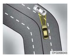
Your vehicle speed can be reduced due to a vehicle in the adjacent lane. Adjust your vehicle speed by depressing the brake pedal according to the road and driving conditions ahead. Apply the accelerator pedal and select the appropriate set speed. Check to be sure that the road conditions permit safe operation of the smart cruise control system.
