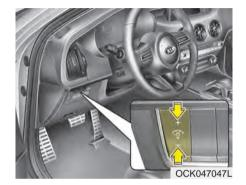
The brightness of the instrument panel illumination is changed by pressing the illumination control button ("+" or "-") when the Engine Start/Stop button is ON, or the taillights are turned on.
