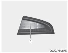
If the rear turn signal lamp (LED) (1), does not operate, have the vehicle checked by an authorized Kia dealer. The LED lamps cannot be replaced as a single component because they are part of an integrated unit. The LED lamps have to be replaced with
