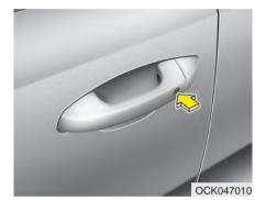
Pressing the button of the front outside door handles with all doors closed and any door unlocked, locks all the doors. The hazard warning lights will blink and the chime will sound once to indicate that all doors are locked. The button will only operate when the smart key is within 28~40 in. (0.7~1 m) from the outside door handle. If you want to make sure that a door has locked or not, you should check the door lock button inside the vehicle or pull the outside door handle.
