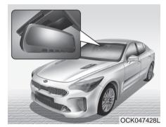
Auto defogging reduces the probability of fogging up the inside of the windshield by automatically sensing the moisture of inside the windshield.
