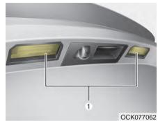
If the license plate lamp (LED) (1) does not operate, have the vehicle checked by an authorized Kia dealer. The LED lamps cannot be replaced as a single component because they are part of an integrated unit. The LED lamps have to be replaced with
