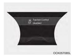
To cancel ESC operation, press the ESC OFF button (ESC OFF \$\frac{1}{20}\$) shortly (ESC OFF indicator light (ESC OFF \$\frac{1}{20}\$) illuminates). At this state, the engine control function does not operate. It means the traction control function does not operate. Brake control function only operates.
