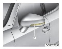
If the side repeater lamp (LED) (1) does not operate, have the vehicle checked by an authorized Kia dealer.
