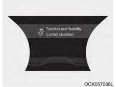
To cancel ESC operation, press the ESC OFF button (ESC OFF ) for more than 3 seconds. ESC OFF indicator light (ESC OFF ) illuminates and ESC OFF warning chime will sound. At this state, the engine control function and brake control function do not operate. It means the car stability control function does not operate any more.
