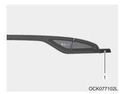
If the rear side marker (LED) (1) does not operate, have the vehicle checked by an authorized Kia dealer. The LED lamps cannot be replaced as a single component because they are part of an integrated unit. The LED lamps have to be replaced with the unit
