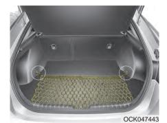
To keep items from shifting in the cargo area, you can use the holders located in the cargo area to attach the luggage net.
