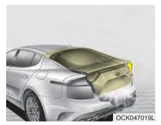
If, during power opening or closing, the liftgate is blocked by an object or part of someone's body, the power liftgate will detect the resistance and it will stop movement or move to the full open position to allow the object to be cleared
