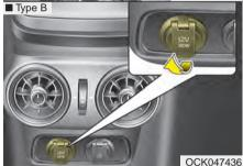
The power outlet is designed to provide power for mobile devices.
