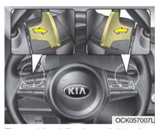
The paddle shifter is available when the shift lever is in the D position or the manual mode.
