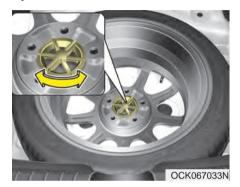
Turn the tire hold-down wing bolt counterclockwise.
