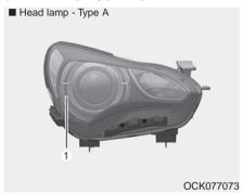
If the position lamp + DRL (LED) (1) does not operate, have the vehicle checked by an authorized Kia dealer.
