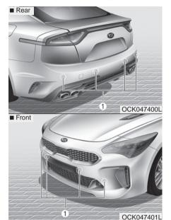
The parking distance warning-forward assists the driver during movement of the vehicle by chiming if any object is sensed within the distance of 39 in. (100 cm) in front and 47 in. (120 cm) behind the vehicle.
