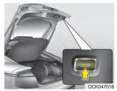
• Press the power liftgate close button for approximately one second when the liftgate is opened.
