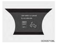
Use switch or pedal to accelerate
