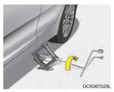
Insert the wheel lug nut wrench into the jack and turn it clockwise, raising the vehicle until the tire just clears the ground. This measurement is approximately 1 in. (30 mm).
