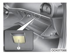
If the glove box lamp (LED) (1) does not operate, have the vehicle checked by an authorized Kia dealer.
