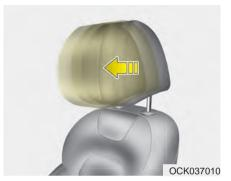
The headrest may be adjusted forward to 4 different positions by pulling the headrest forward to the desired detent
