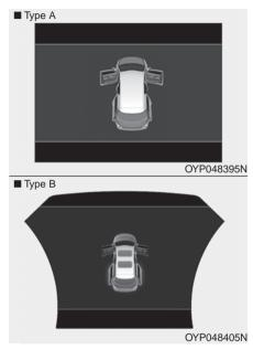
• It means that any door, hood, or liftgate is open.
