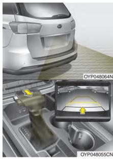
The rear view monitor will activate with the ignition switch ON and the shift lever in the R (Reverse) position.
