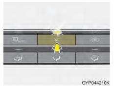
Press the A/C button to turn the air conditioning system on (indicator light will illuminate). Press the button again to turn the air conditioning sys-
