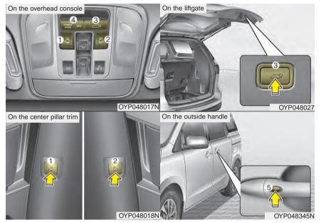
The power sliding doors and power liftgate can be opened and closed automatically with the folding key or smart key, the main control buttons on the overhead console or the sub control buttons on the center pillar trim and the liftgate.
