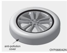
• If the flat tire is contaminated, cover the tire with anti-pollution cover before keeping it indoors. This is to prevent indoor contamination.
