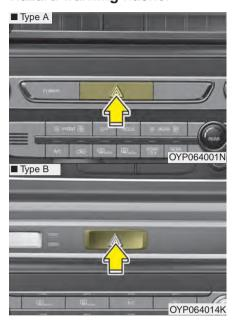
The hazard warning flasher serves as a warning to other drivers to exercise extreme caution when approaching, overtaking, or passing your vehicle. It should be used whenever emergency repairs are being made or when the vehicle is stopped near the edge of a roadway.
