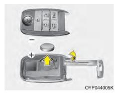
A smart key battery should last for several years, but if the smart key is not working properly, try replacing the battery with a new one. If you are unsure how to use your smart key or replace the battery, contact an authorized Kia dealer.
