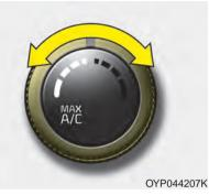
The temperature control knob allows you to control the temperature of the air flowing from the ventilation system. To change the air temperature in the passenger compartment, turn the knob to the right position for warm and hot air or left position for cooler air.
