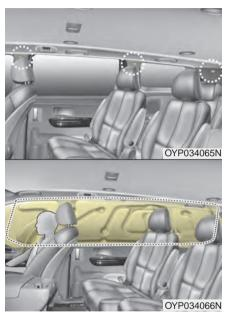
Curtain air bags are located along both sides of the roof rails above the front and rear doors. They are designed to help protect occupants in certain side impacts and to help prevent them from ejecting out of the vehicle as a result of a rollover, especially when the seatbelts are also in use.
