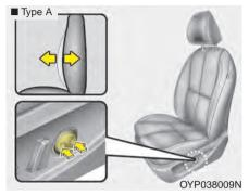
The lumbar support can be adjusted by pressing the lumbar support switch on the side of the drivers seat.
