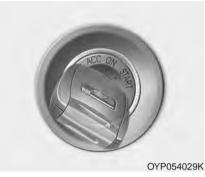
The steering wheel locks to protect against theft (if equipped). The ignition key can be removed only in the LOCK position.
