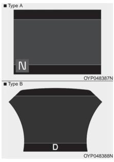
This indicator displays which automatic transaxle shift lever is selected.
