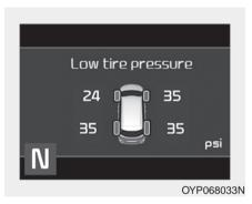
When the tire pressure monitoring system warning indicators are illuminated, one or more of your tires is significantly under-inflated.
