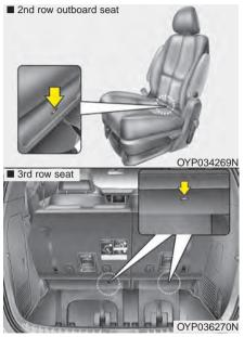
Child restraint hook holders are located on the back of the rear cushions.
