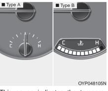
This gauge indicates the temperature of the engine coolant when the ignition switch or Engine Start/Stop button is ON. If the gauge pointer moves beyond the normal range area toward the "H" position, it indicates overheating that may damage the engine.
