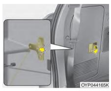
If the fuel filler lid does not open using the remote fuel filler lid release, you can open it manually by pulling the handle outward slightly.
