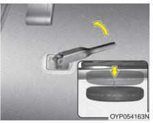
3. Use the wheel lug nut wrench to loosen the bolt enough to lower the spare tire.
