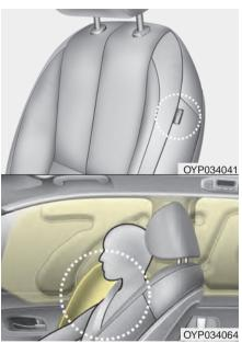
Your vehicle is equipped with a side air bag in each front seat. The purpose of the air bag is to provide the vehicle's driver and/or the front passenger with additional protection than that offered by the seat belt alone.
