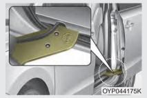
When getting in and out of the sliding door, do not step on the sliding door hinge or drop or put heavy objects on the hinge. The door may not open or close normally by damaging the door hinge or wire part.
