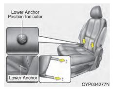
Child restraint symbols are located on the 2nd row outboard seat backs and 3rd row right seat back to indicate the position of the lower anchors for child restraints.
