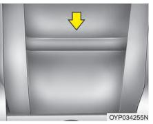
The seatback pocket is provided on the back of the 2nd row outboard seatbacks.
