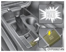
1.Depress the brake pedal, start the engine and then press the Auto Hold button. The white AUTO HOLD indicator will come on indicating the system is in standby.
