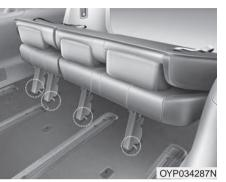
3. Make sure the catches are locked in position by moving the seat forward and backward or lifting the front portion of the seat. If the seat moves, it is not locked properly.
