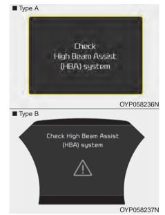
When the High Beam Assist is not working properly, the warning message will come on for a few second. After the message disappears, the master warning light  $(\bigstar)$  will illuminate.
