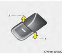
The driver's door has a master power window switch that controls all the windows in the vehicle.
