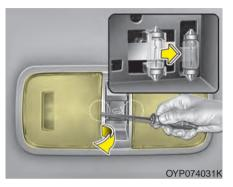
WARNING - Interior lights Prior to working on the Interior lamps, ensure that the "OFF" button is depressed to avoid burning your fingers or receiving an electric shock.
