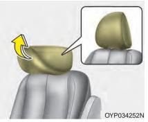
The headrest will fold down automatically when the seat is in the walk in potion.
