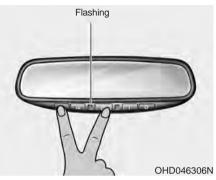
When programming the buttons for the first time, press and hold the left and center buttons (⊉, ££) simultaneously until the indicator light begins to flash after approximately 20 seconds. (This procedure erases the factory-set default codes. Do not perform this step when programming the additional HomeLink buttons.)
