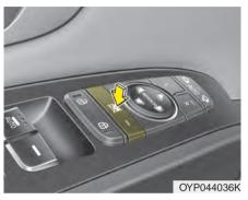
The driver can disable the power window switches on a rear passenger door and the rear sunroof switch on a rear passenger room lamp by depressing the power window and rear sunroof lock switch on the driver's door to LOCK (pressed).
