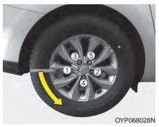
6.Loosen the wheel lug nuts counterclockwise one turn each, but do not remove any nut until the tire has been raised off the ground.
