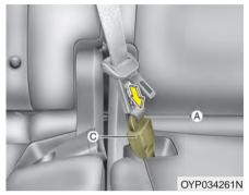
3.Insert the mini tongue (A) into the open end of the anchor connector (C) until an audible "click" is heard, indicating the latch is locked. Make sure the belt is not twisted.
