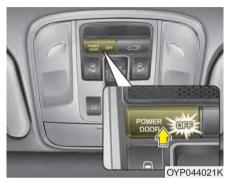
When the power door ON/OFF button is ON (not depressed), the power sliding door and power liftgate can be controlled with the sub control buttons on the center pillar trim or liftgate. Also, the doors can be opened and closed automatically by pulling the inside or outside door handles. • When the power door ON/OFF button is OFF (depressed), the power sliding door and power liftgate can not be controlled with the sub control buttons or door handles.
