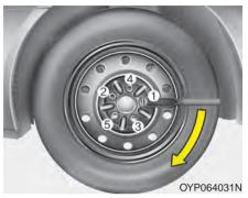
Then position the wrench as shown in the drawing and tighten the wheel nuts. Be sure the socket is seated completely over the nut. Do not stand on the wrench handle or use an extension pipe over the wrench handle. Go around the wheel tightening every nut following the numerical sequence shown in the image until they are all tight. Then double-check each nut for tightness. After changing wheels, have an authorized Kia dealer tighten the wheel nuts to their proper torque as soon as possible.
