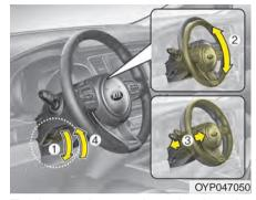
To change the steering wheel angle, pull down the lock-release lever (1), adjust the steering wheel to the desired angle (2) and height (3) then pull up the lock-release lever (4) to lock the steering wheel in place. Be sure to adjust the steering wheel to the desired position before driving.
