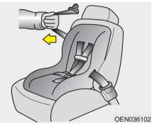
3. Pull the shoulder portion of the seat belt all the way out. When the shoulder portion of the seat belt is fully extended, it will shift the retractor to the "Auto Lock" (child restraint) mode.
