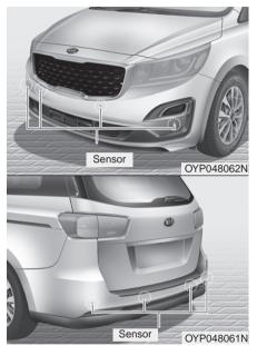
The parking distance warning is not a substitute for proper and safe parking and backing-up procedures. Always drive safely and use caution when parking. The parking distance warning may not detect every object behind or in front of the vehicle. The parking distance warning assists the driver during movement of the vehicle by chiming if any object is sensed within the distance of 39 in (100 cm) in front or behind the vehicle.
