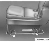
If the rear catches of the seat are locked into the rear anchors (2) while the front catches are not locked into the front anchors (1), do the followings to release the rear catches from the rear anchors
