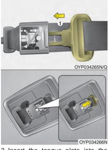
3. Insert the tongue plate into the holder (1) in seat belt and then insert the mini tongue into the hole on the belt assembly cover.
