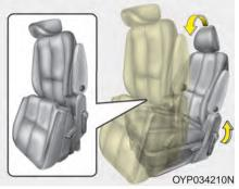
3.At this time, 2nd row seat position will be changed to stand up position, and the head rest will be folded automatically.
