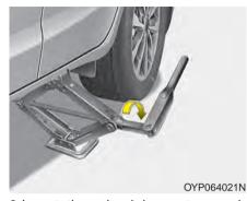
8.Insert the wheel lug nut wrench into the jack and turn it clockwise, raising the vehicle until the tire just clears the ground. This measurement is approximately 1 in. (30 mm).
