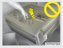
Do not stow the 3rd row seat when the seat back is folded down. It may damage the 3rd seat mechanism.
