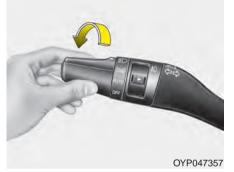
When the light switch is in the headlight position, the head, tail, license lights will turn ON.
