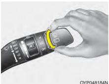
The rear window wiper is switched on automatically when the ignition is in OFF and the gear is shifted to R (Reverse) while the wiper is in motion
