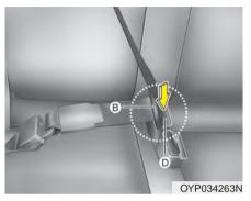
1.Press the release button on the buckle (D) and remove the tongue plate (B) from the buckle (D).
