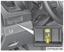
The indicator on the switch will illuminate when the Blind-Spot Collision Warning System (BCW) switch is pressed with the engine start/stop Button ON.
