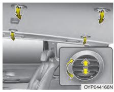
The vent can be adjusted by rotating the blade.
