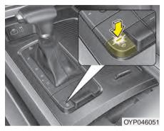
With the ignition switch in the ON position, pressing the heated steering wheel button warms the steering wheel. The indicator on the button will illuminate and notify you on the LCD display. (if equipped)
