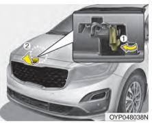
2. Go to the front of the vehicle, raise the hood slightly, pull up the secondary latch (1) inside of the hood center and lift the hood (2).
