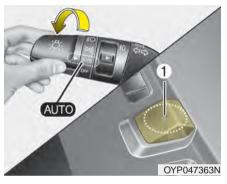
Dynamic bending light uses the steering angle and vehicle speed, to keep your field of vision wide by swiveling the headlamp.
