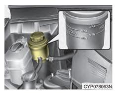
With the vehicle on level ground, check the fluid level in the power steering reservoir periodically. The fluid should be between MAX and MIN marks on the side of the reservoir at the normal temperature.
