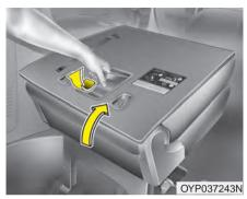
2. Release the lever and push the seat forward firmly until it clicks into place to insert the catches into the anchors.
