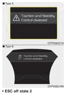
To cancel ESC operation, press the ESC OFF button (ESC OFF 3) for more than 3 seconds. ESC OFF indicator light (ESC OFF 3) illuminates and ESC OFF warning chime will sound.
