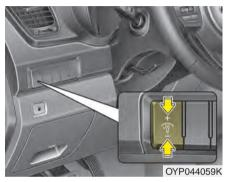
The brightness of the instrument panel illumination is changed by pressing the illumination control button ("+" or "-") when the ignition switch or Engine Start/Stop button is ON, or the tale lights are turned on.
