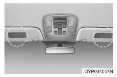
Always have the ignition off when your vehicle is being towed. The side air bags may inflate if the vehicle is tilted such as when being towed because of the rollover sensors in the vehicle. Air bag warning labels, some required by the U.S. National Highway Traffic Safety Administration (NHTSA), are attached to the sunvisor to alert the driver and passengers of potential risks of the air bag system.
