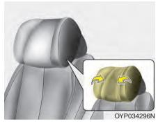
For rear outboard passenger's comfort, the ends of the headrest can be adjusted inward.
