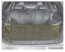
To keep items from shifting in the cargo area, you can use the holders located in the cargo area to attach the luggage net.
