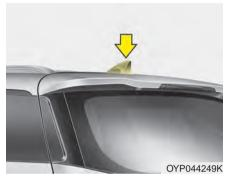
The shark fin antenna will receive the AM, FM broadcast signals and transmit data.
