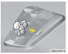
If an object or part of the body is detected while the sunroof is closing automatically, it will reverse direction, and then stop.
