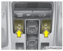
• Push the corresponding main control button on the overhead console to open or close the power sliding door.
