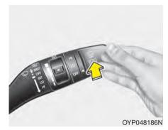
Push the lever away from you to sprav rear washer fluid and to run the rear wipers 1~3 cycles. The spray and wiper operation will continue until you release the lever
