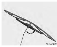
**CAUTION -** Wiper arms Do not allow the wiper arm to fall against the windshield, since it may chip or crack the windshield.
