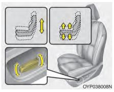
Pull the front portion of the control switch up to raise or press down to lower the front part of the seat cushion. Pull the rear portion of the control switch up to raise or press down to lower the rear part of the seat cushion. Release the switch once the seat reaches the desired position. Walk-in Seat (for front passenger seat, if equipped)
