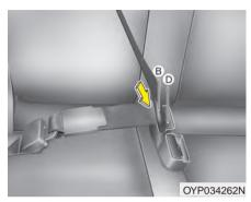
4. Pull the tongue plate (B) and insert the tongue plate (B) into the open end of the buckle (D) until an audible "click" is heard, indicating the latch is locked. Make sure the belt is not twisted.
