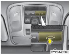
Push the power liftgate main control button for approximately 1 second on the overhead console to open or close the power liftgate. However, the power liftgate will not open with the main control button when all power sliding doors and power liftgate are locked and closed. But the power liftgate will be opened with the folding key (or smart key). • When the power liftgate is operated with the main or sub control button or transmitter, the chime sounds and hazard warning lights flash 2 times.
