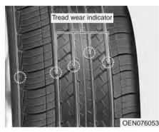
If the tire is worn evenly, a tread wear indicator will appear as a solid band across the tread. This shows there is less than 1/16 inch (1.6 mm) of tread left on the tire. Replace the tire when this happens.
