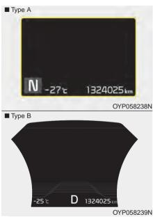
The current outside temperature is displayed in 1°F (1°C) increments. The temperature range is between 40°F ~ 140°F (-40°C ~ 60°C).
