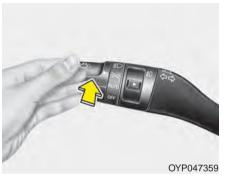
To turn on the high beam headlights, push the lever away from you. The lever will return to its original position.
