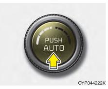
1. Press the AUTO button. The modes, fan speeds, air intake and air-conditioning will be controlled automatically by setting the temperature.
