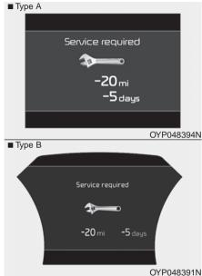
When Service Required is set, the remaining distance/period to drive appears on the LCD screen.
