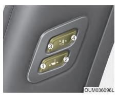
The switch is located on the left side of the front passenger's seatback.
