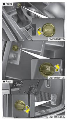
The power outlet is designed to provide power for mobile telephones or other devices designed to operate with vehicle electrical systems. The devices should draw less than 10 amps with the engine running.
