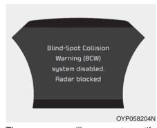
The message will appear to notify the driver if there are foreign substances on the surface or inside the rear bumper or it is hot near the rear bumper. The light on the switch and the system will be turned off automatically.
