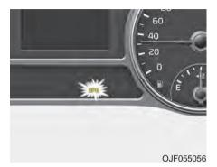
This warning light illuminates if the engine start/stop button is changed to the ON position and goes off in approximately 3 seconds if the system is operationg normally.
