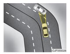
The FCA system may recognize a vehicle in an adjacent lane when driving on a curved road. In this case, the system may apply the brake.
