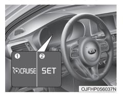
The cruise control system allows you to program the vehicle to maintain a constant speed without depressing the accelerator pedal.
