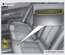
Do not put objects in the center lower part of rear seats. This could block the battery cooling duct causing battery degradation.
