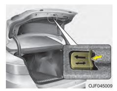
Your vehicle is equipped with an emergency trunk release lever located inside the trunk. If someone is inadvertently locked in the trunk, moving the handle in the direction of the arrow will release the trunk latch mechanism and open the trunk.
