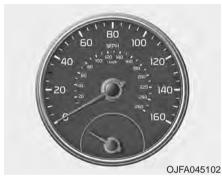
The speedometer indicates the speed of the vehicle and is calibrated in miles per hour (mph) and/or kilometers per hour (km/h).
