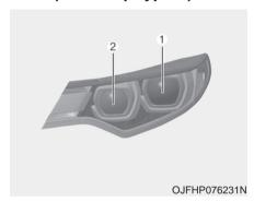
If the head lamp (LED) (1,2) does not operate, have the vehicle checked by an authorized Kia dealer. The LED lamps cannot be replaced as a single component because they are part of an integrated unit. The LED lamps have to be replaced with the unit. A skilled technician should check or repair the head lamp (LED), to avoid damage to related parts of the vehicle.
