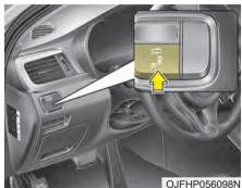
The indicator on the switch will illuminate when the BCW (Blind-Spot Collision Warning) system switch is pressed with the ignition switch ON. If the vehicle speed exceeds 20 mph (30 km/h), the system will activate.
