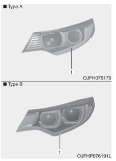
If the position lamp + DRL (1) does not operate, have the vehicle checked by an authorized Kia dealer. The LED lamps cannot be replaced as a single component because they are part of an integrated unit. The LED lamps have to be replaced with the unit. A skilled technician should check or repair the position lamp + DRL (1), to avoid damage to related parts of the vehicle.
