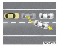
When vehicles are at a standstill and the vehicle in front of you changes to the next lane, be careful when your vehicle starts to move because it may not immediately the stopped vehicle in front of you.
