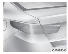
If the stop and tail lamp (LED) does not operate, have the vehicle checked by an authorized Kia dealer. The LED lamps cannot be replaced as a single component because they are part of an integrated unit. The LED lamps have to be replaced with the unit. A skilled technician should check or repair the stop and tail lamp (LED), to avoid damage to related parts of the vehicle.
