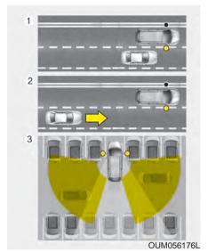
The Blind-Spot Collision Warning (BCW) system uses radar sensors in the rear bumper to monitor and warn the driver of an approaching that it detects in the driver's blind spot area.
