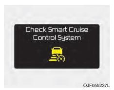
The message will appear when the vehicle to vehicle distance control system is not functioning normally. In this case, take your vehicle to an
