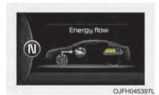
The vehicle is being slowed by engine compression.
