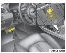
To release the EPB (electronic parking brake), press the EPB switch while doing the following:
