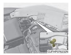
If the charging door does not open due to battery discharge, open the hood and slightly pull the emergency cable which is located in headlamp cover as shown above.
