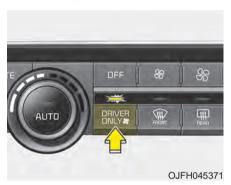
If you press the DRIVER ONLY button( ) and the indicator light illuminates, cold air mostly blows in the direction of the driver's seat. However, some of the cold air may come out of other seats' ducts to keep indoor air pleasant.
