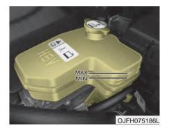
The coolant level should be filled between MAX and MIN marks on the side of the coolant reservoir when the engine is cool.
