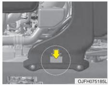
The refrigerant label is located on the top of the air duct assy.
