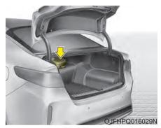
We recommend that the trickle charger cable be put in a storage box after use. Keep the storage box above the main battery pack inside the trunk.
