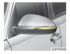
If the side repeater lamp does not operate, have the vehicle checked by an authorized Kia dealer.
