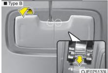
WARNING - Interior lamps Prior to working on the Interior lamps, ensure that the "OFF" button is depressed to avoid burning your fingers or receiving an electric shock.
