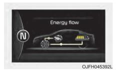
Electric and Engine power are used to move the vehicle.
