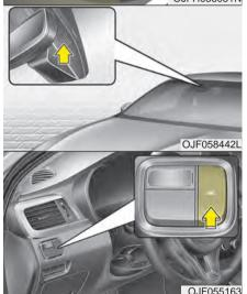
This system is designed to detect the lane in which the vehicle is traveling by using a sensor at the front windshield. In certain situations, the system will warn you when your vehicle is leaving its lane.
