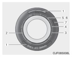
information identifies and This describes the fundamental characteristics of the tire and also provides the tire identification number (TIN) for safety standard certification. The TIN can be used to identify the tire in case of a recall.
