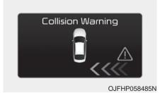
If the vehicle detected by the sensors approaches your vehicle, the warning chime will sound, the warning light on the outside rearview mirror will blink and a message will appear on the LCD display.
