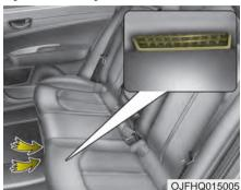
The hybrid battery air intake is located on the bottom of the rear seats. The air intake cools down the hybrid battery.
