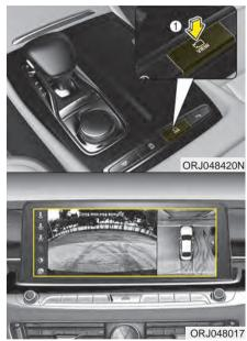
The Surround View Monitoring System (SVM) is not a substitute for proper and safe parking procedures. The Surround View Monitoring System (SVM) may not detect every object surrounding the vehicle. Always drive safely and use caution when parking. The Surround View Monitoring System (SVM) can assist in parking by allowing the driver to see around the vehicle. Push the button (1) into the [ON] position to operate the system.
