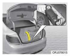
The battery is in the trunk. When replacing the battery, disconnect the negative (-) cable (1) and remove the positive (+) battery fuse box (2).
