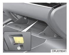
If the glove box lamp (1) does not operate, have the vehicle checked by an authorized K900 Kia dealer.
