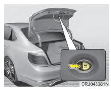
Your vehicle is equipped with an emergency trunk safety release lever located inside the trunk. In the event that someone is inadvertently locked in the trunk, the trunk can be opened by moving the lever in the direction of the arrow and pushing open the trunk.
