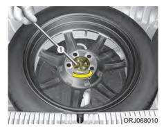
6. Insert the tool (1) into the hole and pull out the wheel cover.
