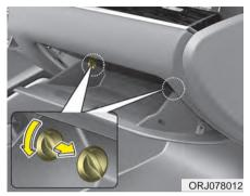
2. Open the glove box and remove the stoppers on both sides.
