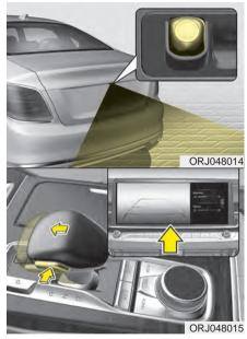
The rear view monitor will activate with the ignition switch ON, engine ON and the shift lever in the R (Reverse) position. This system is a supplemental system that shows the area behind the vehicle on the audio screen while backing up. If the vehicle is equipped with a navigation system, then the system will display the image on the navigation screen. Also, the system displays the area behind the vehicle when the vehicle is in Neutral or Drive if the following conditions are met:
