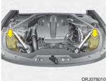
If the vehicle is operated in extremely dusty or sandy areas, replace the element more often than the usual recommended intervals. (Refer to "Maintenance under severe usage conditions" in this chapter.)
