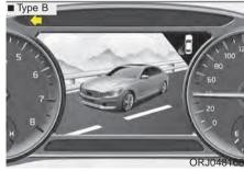
BVM (Blind-spot view monitor) system displays the passenger-side rear areas in the cluster when the system is activated.
