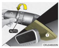
Dynamic Bending Light (DBL) uses the steering angle and vehicle speed, to keep your field of vision wide by swiveling and leveling the headlamp. Change the switch to the AUTO position when the engine is running. The dynamic Bending Light (DBL) will operate when the headlamp is ON. To turn off the DBL, change the switch to other positions. After turning the DBL off, headlamp swiveling no longer occurs, but leveling operates continuously.
