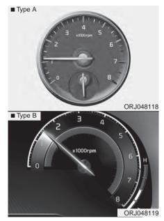
The tachometer indicates the approximate number of engine revolutions per minute (rpm).
