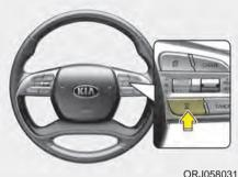
When the Smart Cruise Control system is ON, you can set and maintain the distance to the vehicle ahead without pressing the accelerator or brake pedal.
