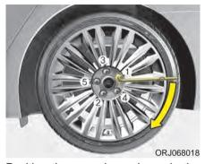
Position the wrench as shown in the drawing and tighten the wheel nuts. Be sure the socket is seated completely over the nut. Do not stand on the wrench handle or use an extension pipe over the wrench handle. Go around the wheel, tightening every nut following the numerical sequence shown in the image until they are all tight. Double-check each nut for tightness. After changing wheels, have an authorized K900 Kia dealer tighten the wheel nuts to their proper torque as soon as possible.
