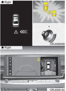
If the vehicle detected by the sensors approaches from the rear left/right side of your vehicle, the warning chime will sound, the warning light on the outside rearview mirror will blink and a message will appear on the LCD display. If the rear view monitor system is in activation, a message will also appear on the AVN screen.
