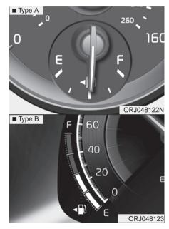
This gauge indicates the approximate amount of fuel remaining in the fuel tank.
