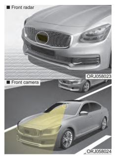
In order for the FCA system to operate properly, always make sure the sensor cover or sensor is clean and free of dirt, snow, and debris. Dirt, snow, or foreign substances on the lens may adversely affect the sensing performance of the sensor.
