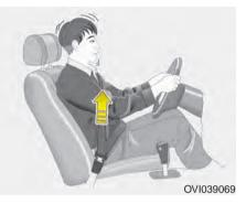
The purpose of the pre-active seat belt is to prevent passengers from getting hurt by tightening the seat belt right before a collision or dangerous maneuver.
