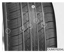
If the tire is worn evenly, a tread wear Indicator (A) will appear as a solid band across the tread. This shows there is less than 1/16 inch (1.6 mm) of tread left on the tire. Replace the tire when this happens.
