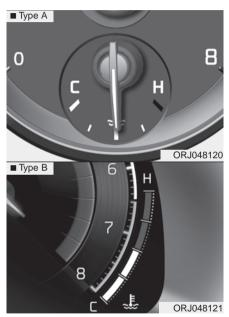
This gauge indicates the temperature of the engine coolant when the Engine Start/Stop button is ON. If the gauge pointer moves or displays beyond the normal range area toward the "H" position, it indicates overheating that may damage the engine.
