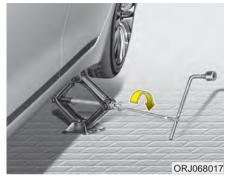
9. Insert the wheel lug nut wrench into the jack and turn it clockwise, raising the vehicle until the tire just clears the ground. This measurement is approximately 1 in. (30 mm).
