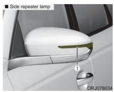
If the side repeater lamp (1) does not operate, have the vehicle checked by an authorized K900 Kia dealer.
