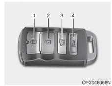
All doors are locked if the lock button is pressed. If all doors (and trunk) are closed, the hazard warning lights will blink once to indicate that all doors
