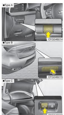
The power trunk can be opened and closed automatically as follows.
