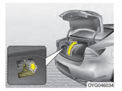
If the fuel filler lid does not open using the fuel filler lid opener button, you can open it manually. Remove the panel in the cargo area. Pull the handle out slightly.
