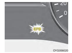
This warning light illuminates if the engine start/stop button is changed to the ON position and goes off in approximately 3 seconds if the sys-
