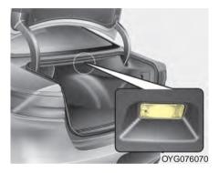
If the trunk lamp (LED) does not operate, have the vehicle checked by an authorized Kia dealer.
