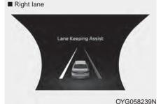
If the vehicle leaves a lane, the lane marker you cross will blink on the LCD display.
