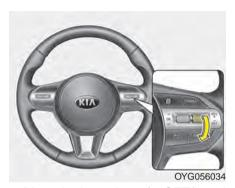
Move the lever down (to SET-), and release it at the desired speed. The cruise indicator and set speed on the LCD screen will illuminate. Release the accelerator at the same time. The desired speed will automatically be maintained.
