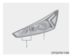
If the head lamp (LED) (1,2) does not operate, have the vehicle checked by an authorized Kia dealer. The LED lamps cannot be replaced as a single unit because it is an integrated unit. The LED lamps has to be
