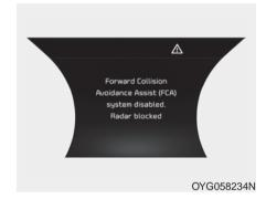
When the sensor is covered or the sensor lens is dirty with foreign substances, such as snow or rain, the FCA system may not be able to detect vehicles or pedestrians. In this case, a warning message
