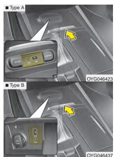
You can use an aux port to connect audio devices and an USB port to plug in an USB or iPod<sup>®</sup>.
