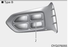
If the front fog lamp (LED) (1, 2) does not operate, have the vehicle checked by an authorized Kia dealer. The LED lamps cannot be replaced as a single unit because it is an integrated unit. The LED lamps has to be replaced with the unit.
