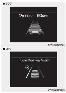
This mode displays the state of the Smart Cruise Control with Stop & Go (SCC) and Lane keeping Assist (LKA) system.
