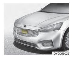
In order for the FCA system to operate properly, always make sure the sensor or sensor cover is clean and free of dirt, snow, and debris. Dirt, snow, or foreign substances on the lens may adversely affect the sensing performance of the sensor.
