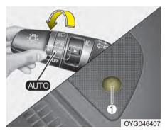
When the light switch is in the AUTO light position, the taillights and headlights will turn ON or OFF automatically depending on the amount of light outside of the vehicle.
