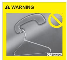
Do not hang other objects such as hangers or hard objects except clothes. Also, do not put heavy, sharp or breakable objects in the pockets of the clothing. In an accident or when the curtain air bag is inflated, it may cause vehicle damage or personal injury.
