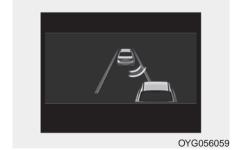
The Blind-Spot Collision-Avoidance Assist System (BCA) may apply braking power, when an approaching vehicle is detected within a certain
