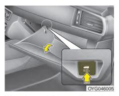
When the trunk lid control button is in UNLOCK, the power trunk can be controlled with the power trunk main control button, power trunk open, close button, and the smart key.
