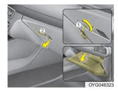
The glove box can be locked and unlocked with a master key (1). (if equipped)
