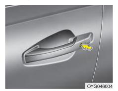
Pressing the button on the front outside door handles with all doors closed and any door unlocked, locks all the doors. The hazard warning lights will blink and the chime will sound once to indicate that all doors are locked. The button will only operate when the smart key is within 28~40 in. (0.7~1 m) from the outside door handle. If you want to make sure that a door has locked or not, you should check the door lock button inside the vehicle or pull the outside door handle.
