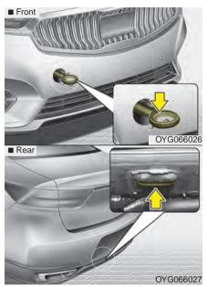
If towing is necessary, we recommend you to have it done by an authorized Kia dealer or a commercial tow truck service. If towing service is not available in an emergency, your vehicle may be temporarily towed using a cable or chain secured to the emergency towing hook under the front (or rear) of the vehicle. Use extreme caution when towing the vehicle. A driver must be in the vehicle to steer it and operate the brakes.
