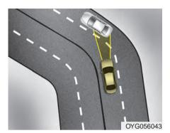
Your vehicle speed can be reduced due to a vehicle in the adiacent lane. Adjust your vehicle speed by depressing the brake pedal according to the road and driving conditions ahead. Apply the accelerator pedal and select the appropriate set speed. Check to be sure that the road conditions permit safe operation of the smart cruise control system.
