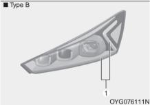
If the position lamp + DRL\* (1) does not operate, have the vehicle checked by an authorized Kia dealer. The LED lamps cannot be replaced as a single unit because it is an integrated unit. The LED lamps has to be replaced with the unit.
