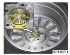
Turn the tire hold-down wing bolt counterclockwise.
