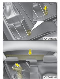
To fold the rear curtain, press the button. To unfold the rear curtain. press the button again.
