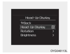
The HUD display may be activated or deactivated in user setting mode while engine is ON.
