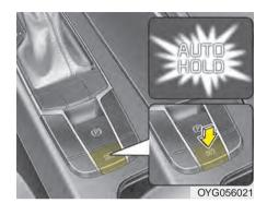
1.Depress the brake pedal, start the engine and then press the Auto Hold button. The white AUTO HOLD indicator will come on indicating the system is in standby. Before the Auto Hold will engage, the driver's door and engine hood must be closed and the driver's
