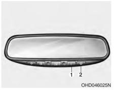
To operate the electric rearview mirror Press the I button (1) to turn the automatic- dimming function on. The mirror indicator light will illuminate.
