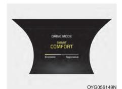
Once the SMART MODE is selected by pressing the DRIVE MODE button, and the DRIVE MODE indicator screen is selected by pressing the trip computer button on the steering wheel, the driving style gauge bar will show up at the bottom of screen
