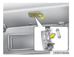
WARNING - Interior lamps Prior to working on the Interior lamps, ensure that the "OFF" button is depressed to avoid burning your fingers or receiving an electric shock.
