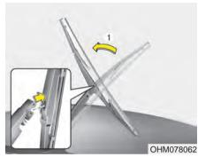
1. Raise the wiper arm and pull out the wiper blade assembly.
