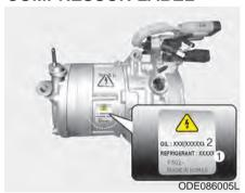
A compressor label informs you the type of compressor your vehicle is equipped with such as model, supplier part number, production number, refrigerant (1) and refrigerant oil (2).
