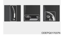
This gauge indicates the remaining hybrid battery power. If the SOC is near the "L (Low)" level, the vehicle automatically operates the engine to charge the battery.
