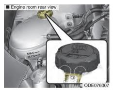
2. Make sure that the tiny protrusions inside the coolant cap should be securely interlocked.
