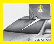
The Aux. Battery Saver+ relies on the high voltage battery to charge the 12V battery. The charging indicator lamp will blink rapidly when this is occurring. To reduce the risk of electrical shock, do not touch any high voltage components (orange) or other electrical devices while charging is occurring.
