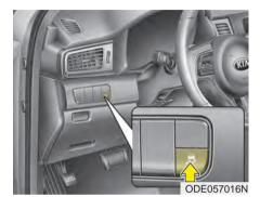
The Electronic Stability control (ESC) system is designed to stabilize the vehicle during cornering maneuvers. ESC checks where you are steering and where the vehicle is actually going. ESC applies the brakes on individual wheels and intervenes with the engine management system to stabilize the vehicle. Electronic stability control (ESC) will not prevent accidents. Excessive speed in turns, abrupt maneuvers and hydroplaning on wet surfaces can still result in serious accidents.
