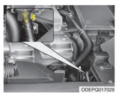
If the charging connector does not unlock for some reason, open the hood and slightly pull the emergency cable as shown above. The charging door will then open.
