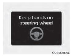
If the driver takes hands off the steering wheel for several seconds while the LKA is activated, the system will warn the driver
