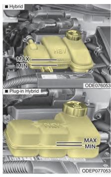
The coolant level should be filled between MAX and MIN marks on the side of the coolant reservoir when the engine is cool.
