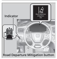
Press the Road Departure Mitigation button to turn the system on and off.
