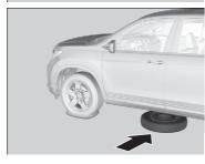
**7.** Place the compact spare tire (wheel side up) under the vehicle body, near the tire that needs to be replaced.
