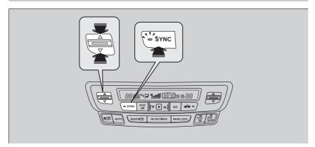
You can set the temperature synchronously for the driver side, front passenger side and rear seats in synchronized mode.
