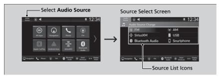
Select **Audio Source** in the header area, then select an icon on the source list to switch the audio source.
