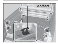
The tie-down anchors on the pickup bed can be used to install a net for securing items.
