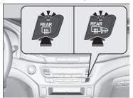
The rear defogger and heated door mirror\* automatically switch off after 10-30 minutes depending on the outside temperature.
