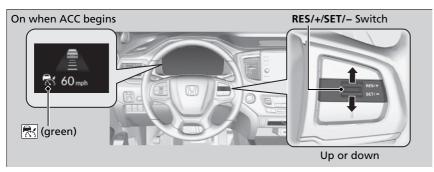
Take your foot off the pedal and press the **RES/+/SET/**– switch up or down when you reach the desired speed. The moment you release the switch, the set speed is fixed, and ACC begins.
