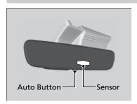
When you are driving after dark, the automatic dimming rearview mirror and power door mirrors\* reduce the glare from headlights behind you. Press the auto button to turn this function on and off. When activated, the auto indicator comes on.
