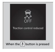
This button is on the driver side control panel. To partially disable VSA® functionality/ features, press and hold it until you hear a beep.
