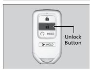
Press the unlock button, and then within 10 seconds, press it again and hold it.
