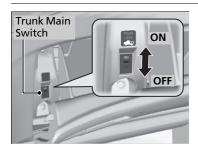
The trunk main switch disables the trunk release button on the trunk lid to protect luggage in the trunk.
