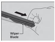
**4.** Slide the wiper blade out of the holder by pulling the tabbed end out.
