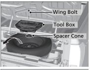
**5.** Unscrew the wing bolt, and remove the tool box and the spacer cone. Then, remove the compact spare tire.
