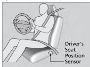
The driver's advanced airbag system includes a seat position sensor.
