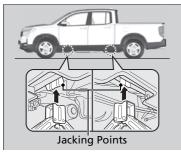
**1.** Place the jack under the jacking point closest to the tire to be changed.
