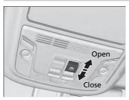
**To open:** Pull the switch back. **To close:** Push the switch forward.
