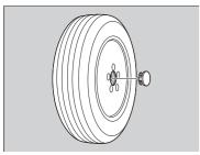
**1.** Remove the center cap and place the tire on the pickup bed.
