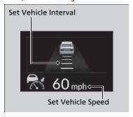
When ACC starts operating, the vehicle icon, interval bars and set speed appear on the driver information interface.
