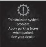
■ Reasons for the indicator to blink The transmission is malfunctioning.
