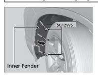
**1.** Turn the steering wheel all the way to the opposite side from the front turn signal/ parking\* light being replaced.
