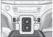
The seat heaters or ventilators can be used when the power mode is in ON.
