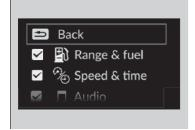
**3.** Roll the left selector wheel to scroll between icons, then press the left selector wheel to check or uncheck them.
