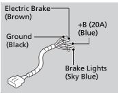
The trailer hitch harness is used to install the controller for the electric trailer brakes. Insert the trailer brake fuse into the engine compartment sub fuse box.
