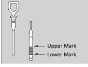
**4.** Remove the dipstick again, and check the level. It should be between the upper and lower marks. Add oil if necessary.
