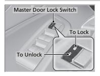
Press the master door lock switch in as shown to lock or unlock all the doors.
