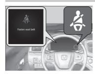
The seat belt system includes an indicator on the instrument panel to remind the driver or a front passenger or both to fasten their seat helts
