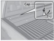
**2.** Wrap a cloth around the tip of a small flattip screwdriver. Put it into the cap as shown in the image, and remove the cap.
