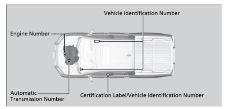
■Vehicle Identification Number (VIN), Engine Number, and Transmission Number
