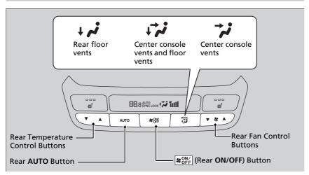
Use the system when the engine is running and the climate control system is operating.
