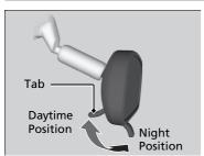
Flip the tab to switch the position.
