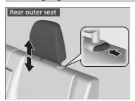
A passenger sitting in the rear seating position should adjust the height of their head restraint to an appropriate position before the vehicle begins moving.
