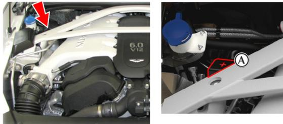
8. Leave the jump start cables attached and the engines running for 2 to 3 minutes to allow the battery to charge.
