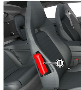
The purpose of the airbags is to provide **additional** protection for the driver and passengers in the event of a serious impact (front or side impacts). The airbags are supplementary to the seat belts.
