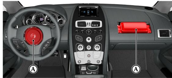
The front airbags (A) only deploy in a serious front collision. The side airbags, located in the front seats (B) and the door top panels (C) only deploy according to which side has been impacted in a serious side collision. The airbags mounted in the door top panels on each door are designed to protect the heads of the driver and passengers during certain side impacts.
