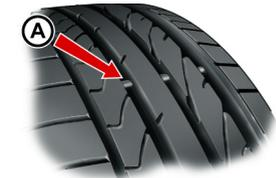
When a tyre has worn causing one or more of the marks to be flush with the outer face of the tread the tyre has reached its wear limit. It then becomes illegal in certain countries and must be replaced.
