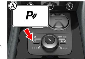
If an obstacle is detected at the front or rear of the vehicle, a series of beeps will be heard from the front or rear speaker respectively, which increases in rate as the vehicle nears the obstacle.
