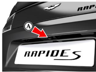
If the infotainment screen is ON when reverse gear is selected the screen will show the camera view until reverse gear is deselected. When reverse gear is deselected the screen will continue to show the camera view for approximately ten seconds or when the vehicle reaches a speed of 16 km/h (whichever is sooner), then return to the infotainment screen.
