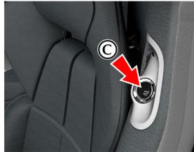
To raise lift the seat back to its upright position, take care not to trap the seat belt, and make sure that the seat back is locked into position (button LED OFF). If the button LED stays ON the seat back is not locked in place.
