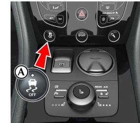
**OFF:** From Track mode, press and hold the DSC button for four seconds and release to set the DSC to OFF. DSC OFF can not be selected from DSC ON. DSC FUNCTION OFF will show in the message centre. DSC is no longer controlling engine torque and applying strategic application of the brakes at individual wheels. At any time while in track or off mode, press and release the DSC button to start DSC.
