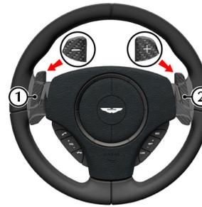
If no gearshift has been requested by pulling back on a paddle, upshifts and downshifts will occur automatically if the engine speed rises or lowers to its maximum or minimum operating limits. This does not occur if the transmission is in sport mode (Refer to 'Sport Mode', page 5.7).
