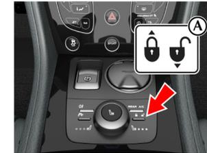
If the vehicle is locked using the master lock switch, one pull of a door handle will centrally unlock the doors and a second pull of the door handle will open that door.
