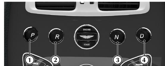
**[1] PARK:** Press and release to select park once the vehicle is stationary. The transmission will mechanically lock. If the vehicle key is moved to position '0' or removed from the ignition control while the vehicle is at a standstill, the transmission will automatically select park.
