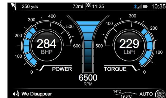
The screen will show both power and torque along with engine speed. On the power and torque dials there will be two readings:
