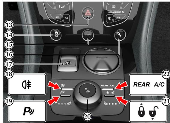
**[13] HAZARD WARNING LAMP:** Press to set the hazard warning lamps to ON or OFF.
