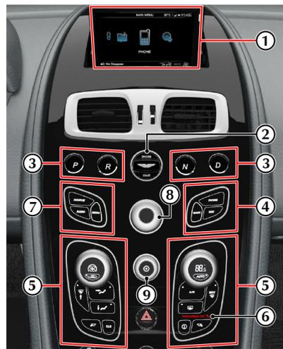
**[1] INFOTAINMENT SCREEN:** Opens when the infotainment system is set to ON.
