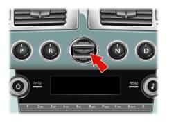
▲ Warning: Only use the vehicle key in the ignition control. Do not place any objects, including fingers, into the ignition control other than the vehicle key. Objects other than the vehicle key may cause the ignition control to fail. V The vehicle key must only be inserted into the ignition control with the two indents first, as shown. Attempting to insert the larger end first the key may damage the ignition control.
