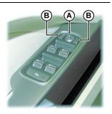
When the heated rear window is ON the heaters in the door mirrors will operate for 6.5 minutes.
