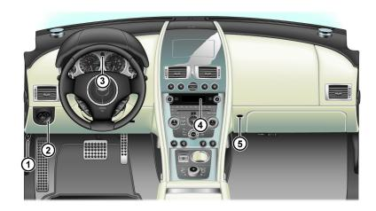
[1] FUEL FLAP RELEASE - Press to open the fuel flap. Close the fuel flap by pressing down on the flap until the lock engages.
