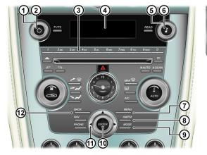
[1] ON/OFF - Press for audio ON and OFF.[2] VOLUME - Volume control.
