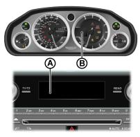
[a] - Warning - Low Battery/Emphasis' (For 10 seconds).[B] - 'Low Battery'.
