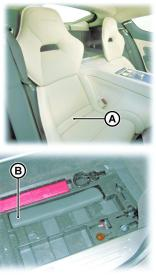
Secure the child seat using the LATCH lower anchors, following the child seat manufacturer's instructions. **Tether Anchor**
