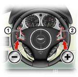
If no gearshift has been requested by pulling back on a paddle, upshifts and downshifts will occur automatically if the engine speed rises or lowers to its maximum or minimum operating limits (unless the transmission is in sport mode (Refer to 'Sport Mode', page 5.6)).
