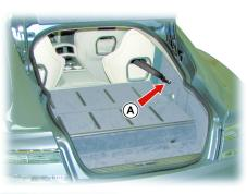
Route the tether strap through the seat back as shown. Engage the tether clip to the anchor point as shown and make sure that the locking spring has fully closed to prevent accidental disengagement. Always make sure that the tether strap length is adjusted to remove any slack.
