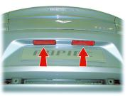
The trunk illumination comprises of four LEDs, two each side of the trunk area and are not repairable.
