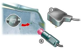
To remove the battery conditioner first disconnect from the mains supply, then from the vehicle socket.
