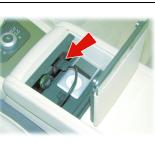
Music devices connected using the 3.5 mm jack socket will not be operated by the vehicle audio system or have their batteries charged (Refer to 'Auxiliary Functions', page 7.16).
