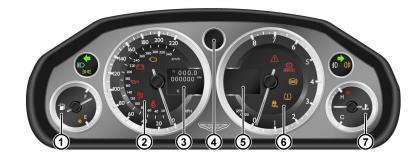
[4] GEAR POSITION INDICATOR - Shows the current transmission position when in Auto Drive mode and the current gear selection when in Touchtronic mode (Refer to 'Automatic Transmission', page 5.3).
