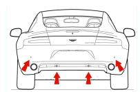
V In heavy rain or similar adverse conditions, the rear parking assist sensors may not always be able to accurately measure distance to close objects. A fully laden vehicle or irregular obstacles may also cause inaccurate measurements. The parking assist system defaults to OFF when the ignition is set to ON. The system comes ON when reverse gear is selected, or if the parking assist button (A) is pressed at speeds below 15 km/h (9 mph).
