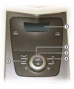
[1] DISPLAY - Shows the fan speed or temperature when selected.
