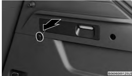
Fuel Door Emergency Release
