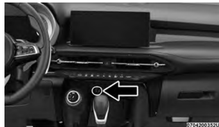
Power Outlet Location
