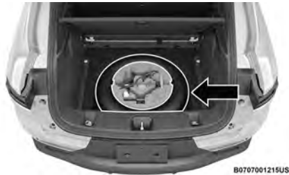
Damaged Tire Storage
