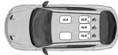
Switchable Automatic Locking Retractor (ALR) Locations
