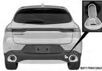
Rear Tow Eye Installed
