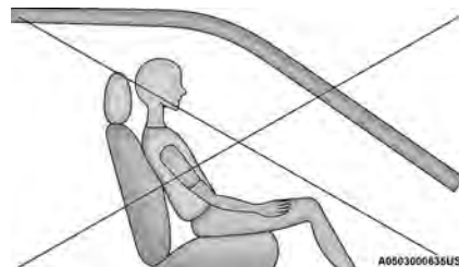
Not Seated Properly
