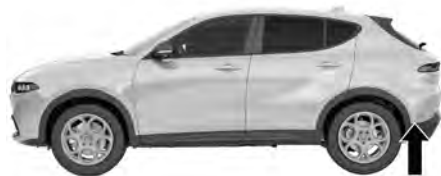
Radar Sensor Location (Driver Side Shown)
