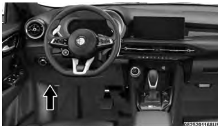
Interior Fuse Box Location
