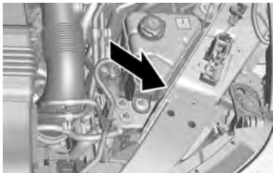
Protective Cover Location
