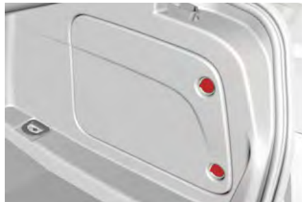
Battery Access Panel
