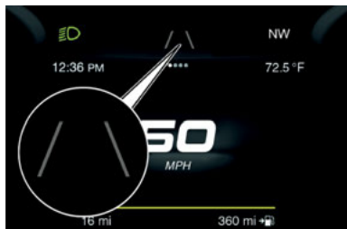
Lane Markings Not Detected
