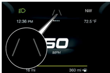
Lane Markings Not Detected
