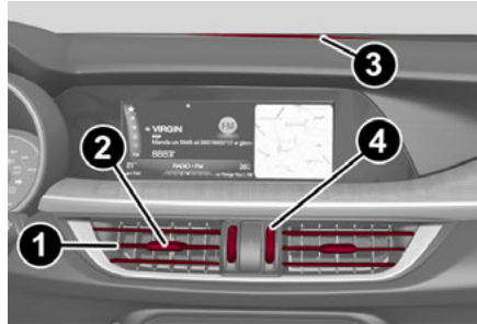
Central Air Vents
