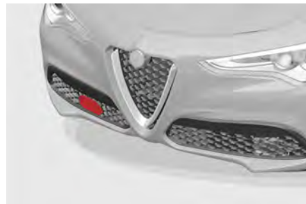
Front Fascia/Bumper Radar Location
