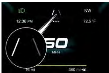
Left Lane Marking Detected
