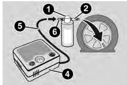
Attaching Filler Tube To Deflated Tire
